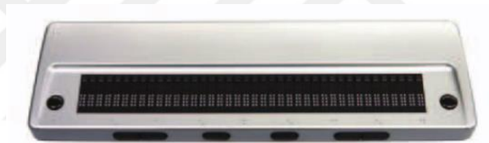
Figure 1.26 Linear refreshable braille display (Maham et al., 2016)
