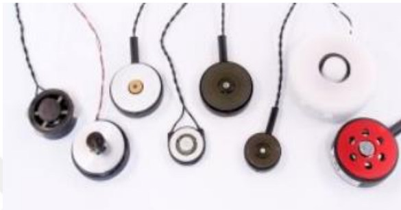
Figure 1.20 Some types of tactors (EAI Engineering Acoustic Inc., n.d.)
