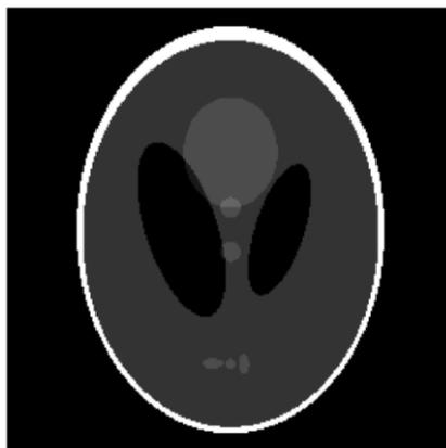
Figure 5.6 The image reconstructed by SENSE had no problem when the number of coils is sixteen and the acceleration factor is four
