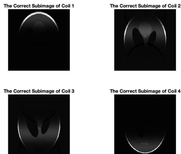
Figure 4.14 Sensitivity map for each receiver coil
