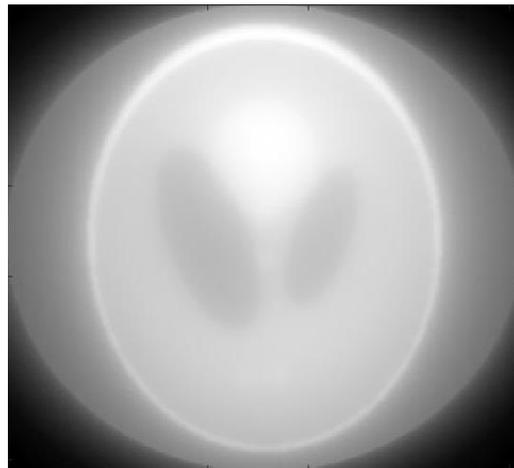
Figure 4.7 Final image of back-projection method for 2D sample
