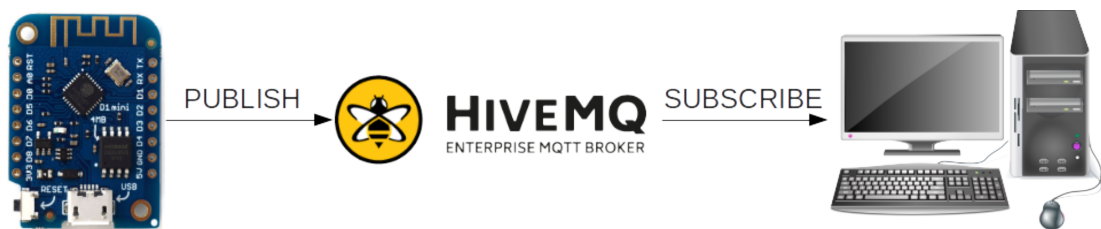
Figure 4.1 D1 Mini (D1 Mini Image, n.d.), is publishing a data packet to a topic in MQTT Dashboard (HiveMQ Logo, n.d.). Simultaneously, a computer (Desktop PC Image, n.d.) has subscribed to the same topic that D1 Mini is sending data and receives this data from MQTT Dashboard
