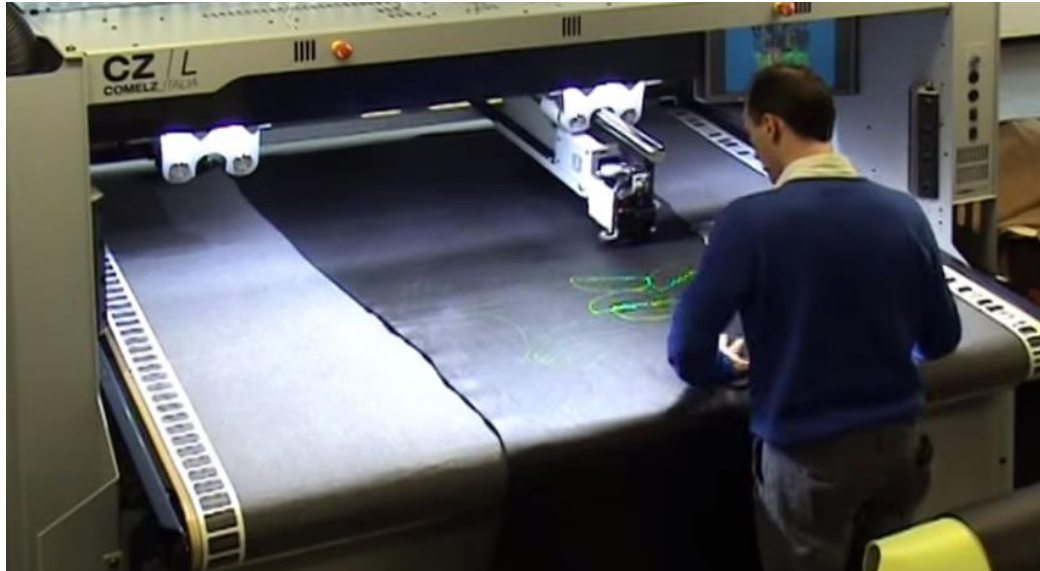
Figure 1.2 CNC Leather Cutter that a kind of CNC Router
