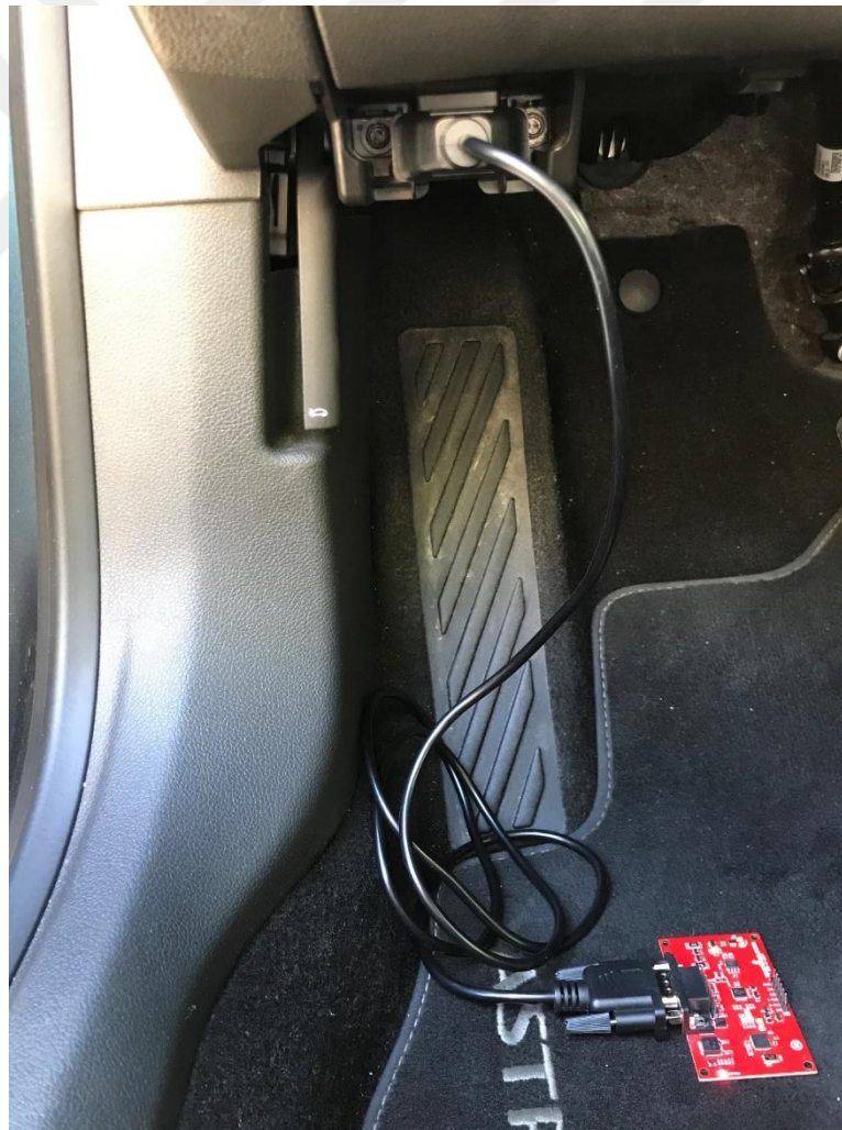
Figure 4.1 OBD port connection (Personal archive, 2019)
