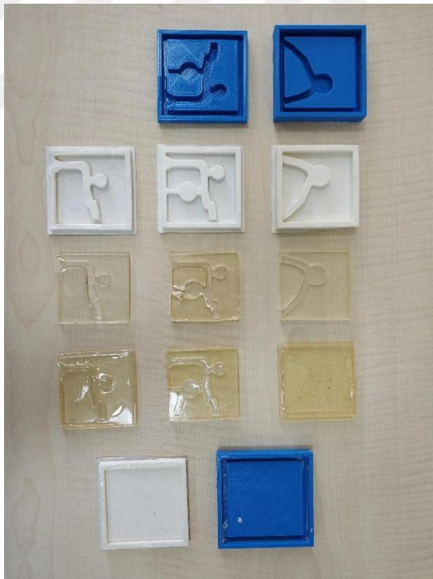
Figure 6.17 The resin models and their silicon moulds for  $xz$  motion
