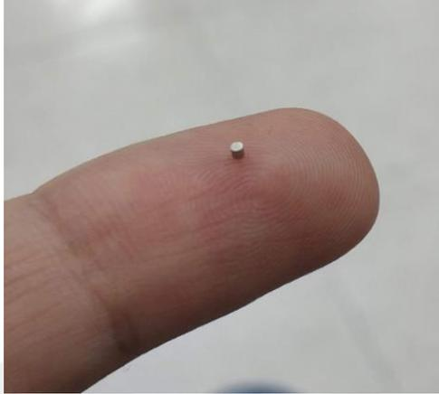
Figure 2.5 N35 grade cylindrical permanent magnet with 1 mm to 1 mm dimensions (Kahveci et al., 2021)
