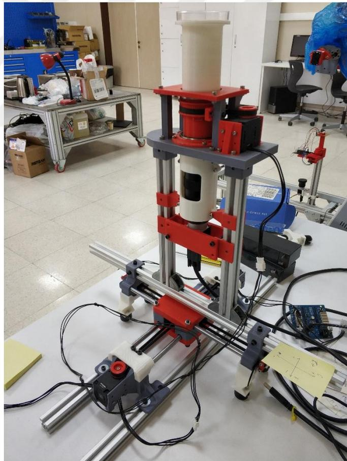
Figure 4.15 Manufactured subsidiary manipulator system
