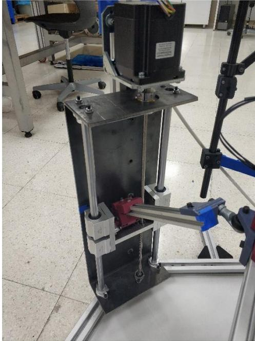
Figure 4.11 Design improvement with major structure reinforcement revisions with leg and spherical joint structure
