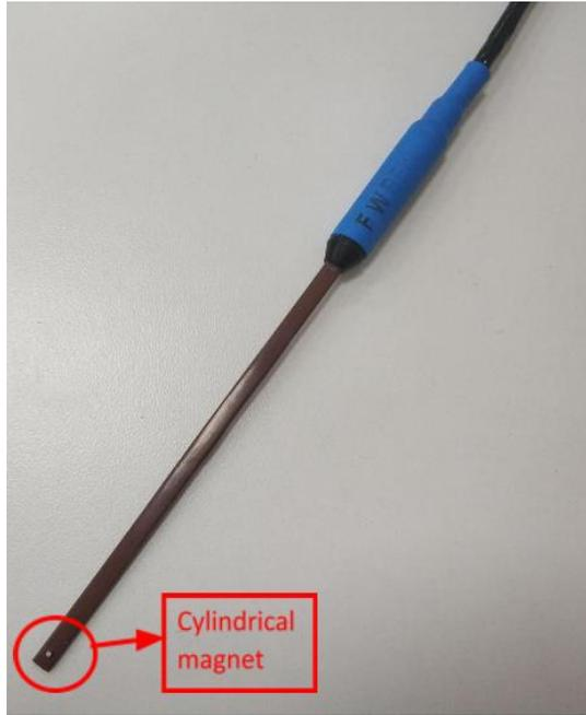
Figure 2.9 The positioning of the permanent magnet on the probe
