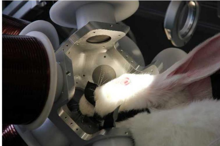
Figure 1.15 Microrobot test in rabbit eye placed into OctoMag setup (Ullrich et al., 2013)
