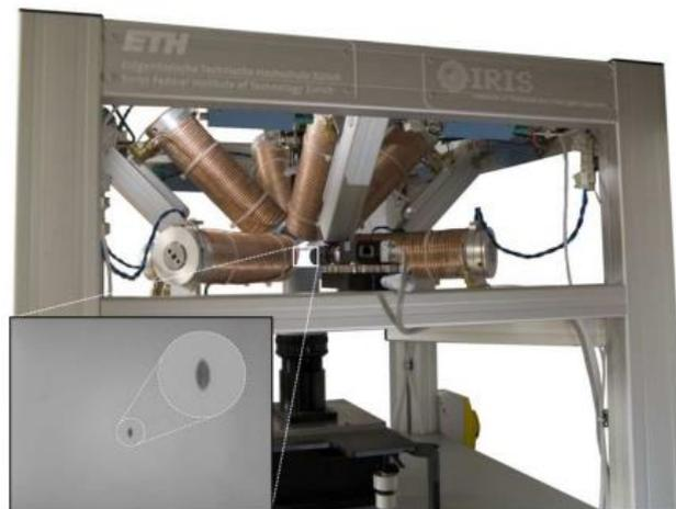
Figure 1.6 OctoMag setup (Kummer et al., 2010)
