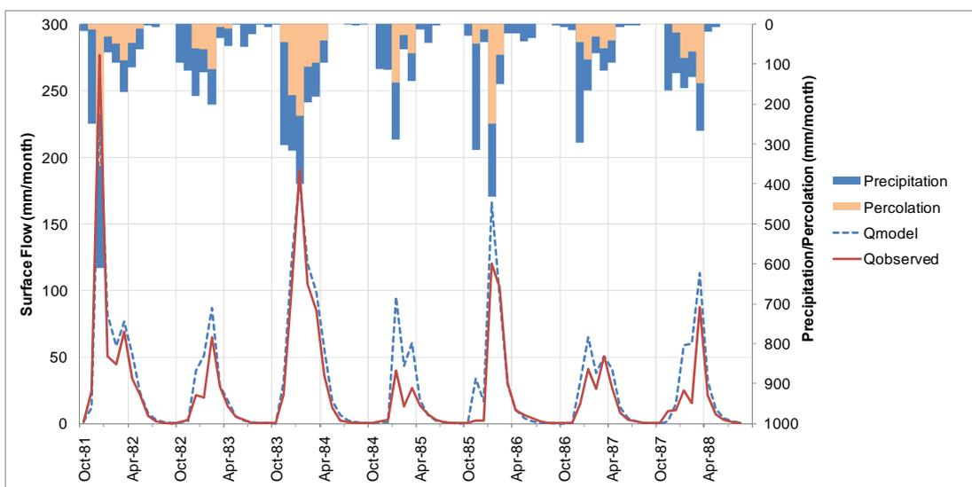
Figure 6.2 Results of the precipitation-runoff model; hydrographs for the verification period
