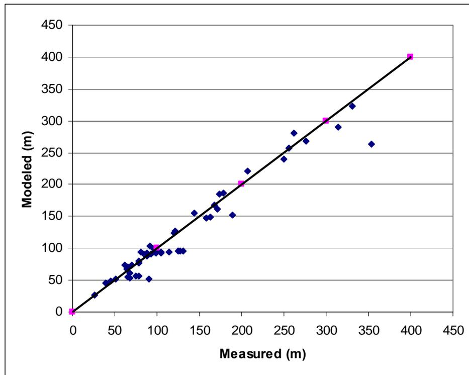
Figure 6.4 Comparison of modeled with measured head values for the uncalibrated model
