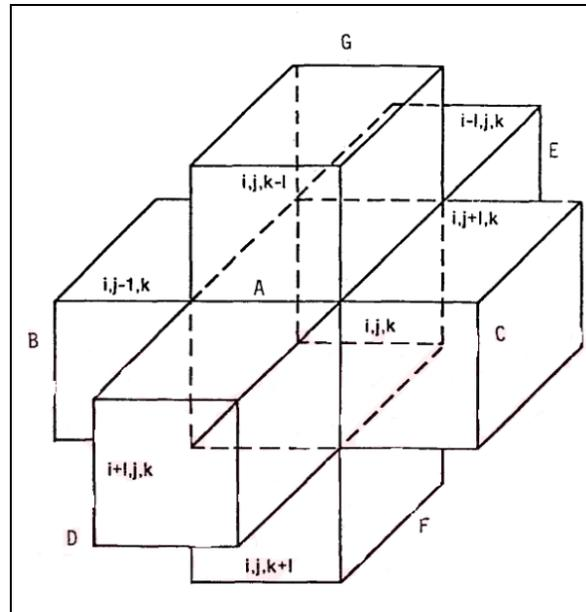
Figure 1.3 Illustration of a finite-difference computational molecule
