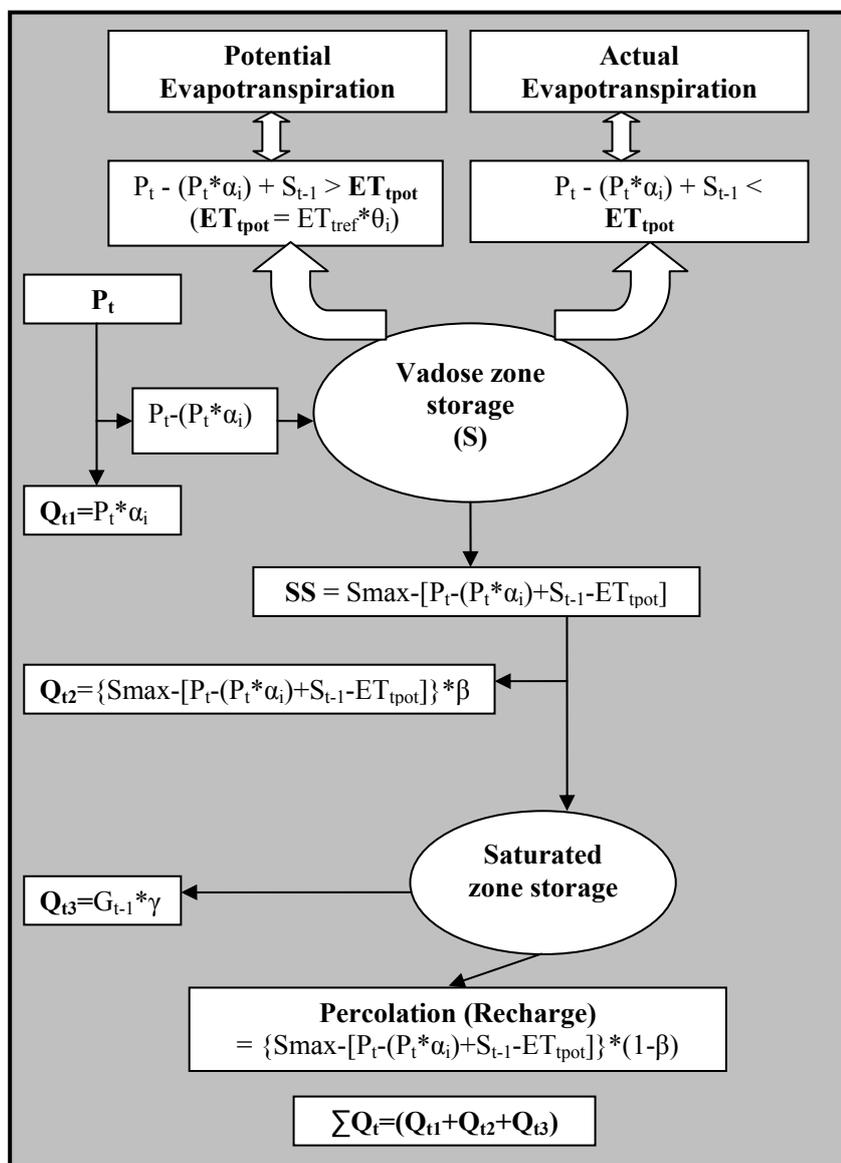
Figure 4.6 Components and flow chart of the water budget based precipitation-runoff model (adapted from Fıstıkođlu & Harmancıođlu (2001))
