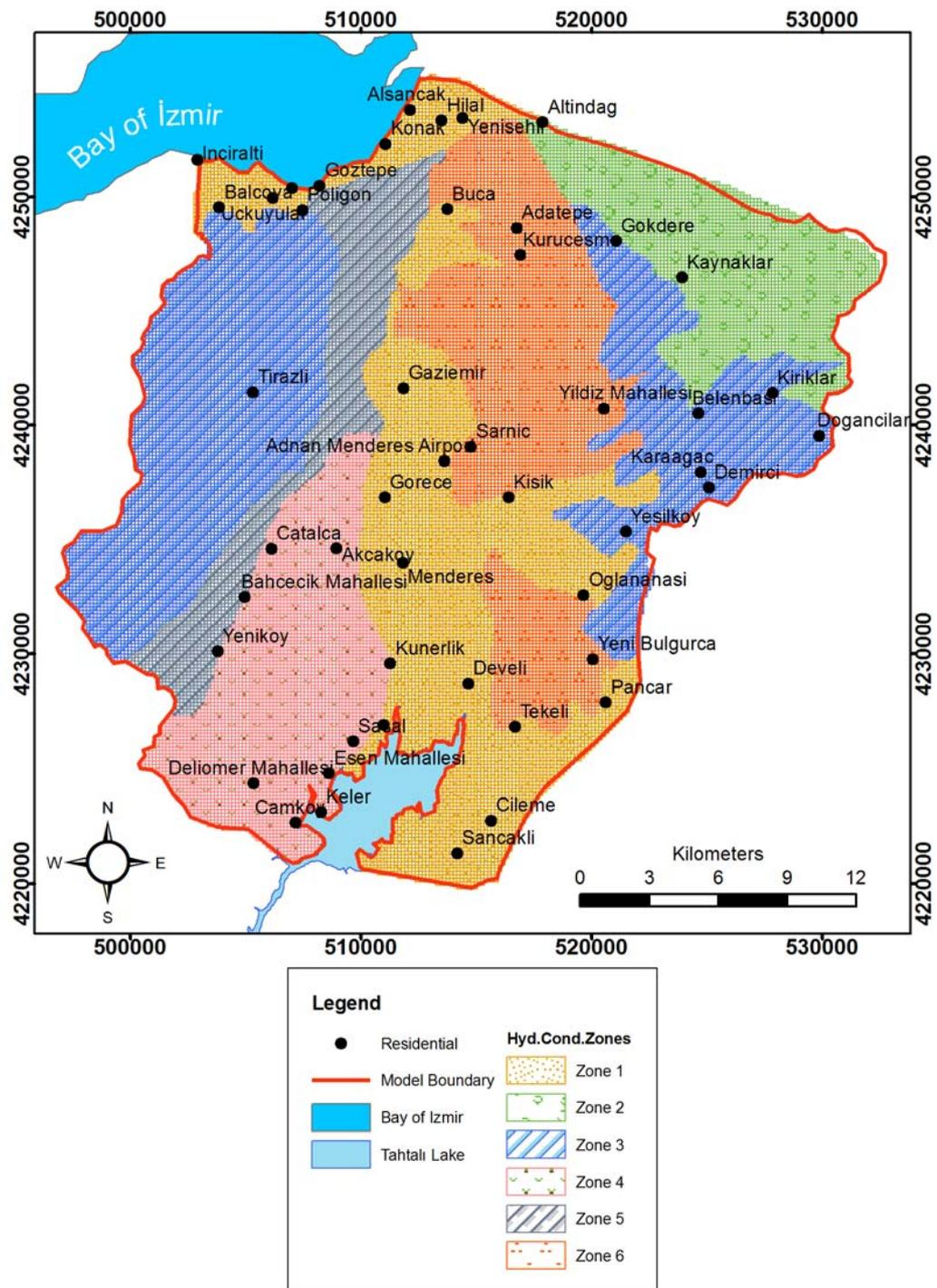
Figure 5.2 Hydraulic conductivity zones used in the model
