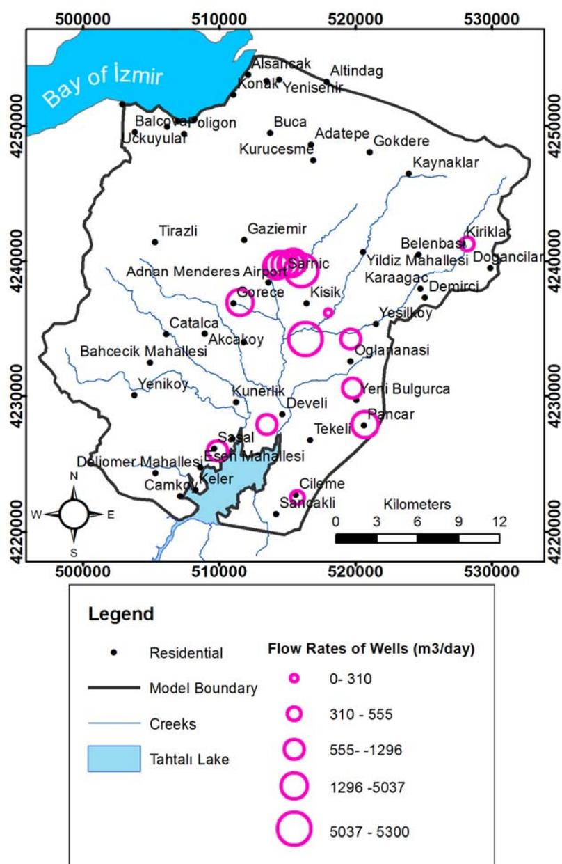
Figure 5.4 Water supply wells included in the model
