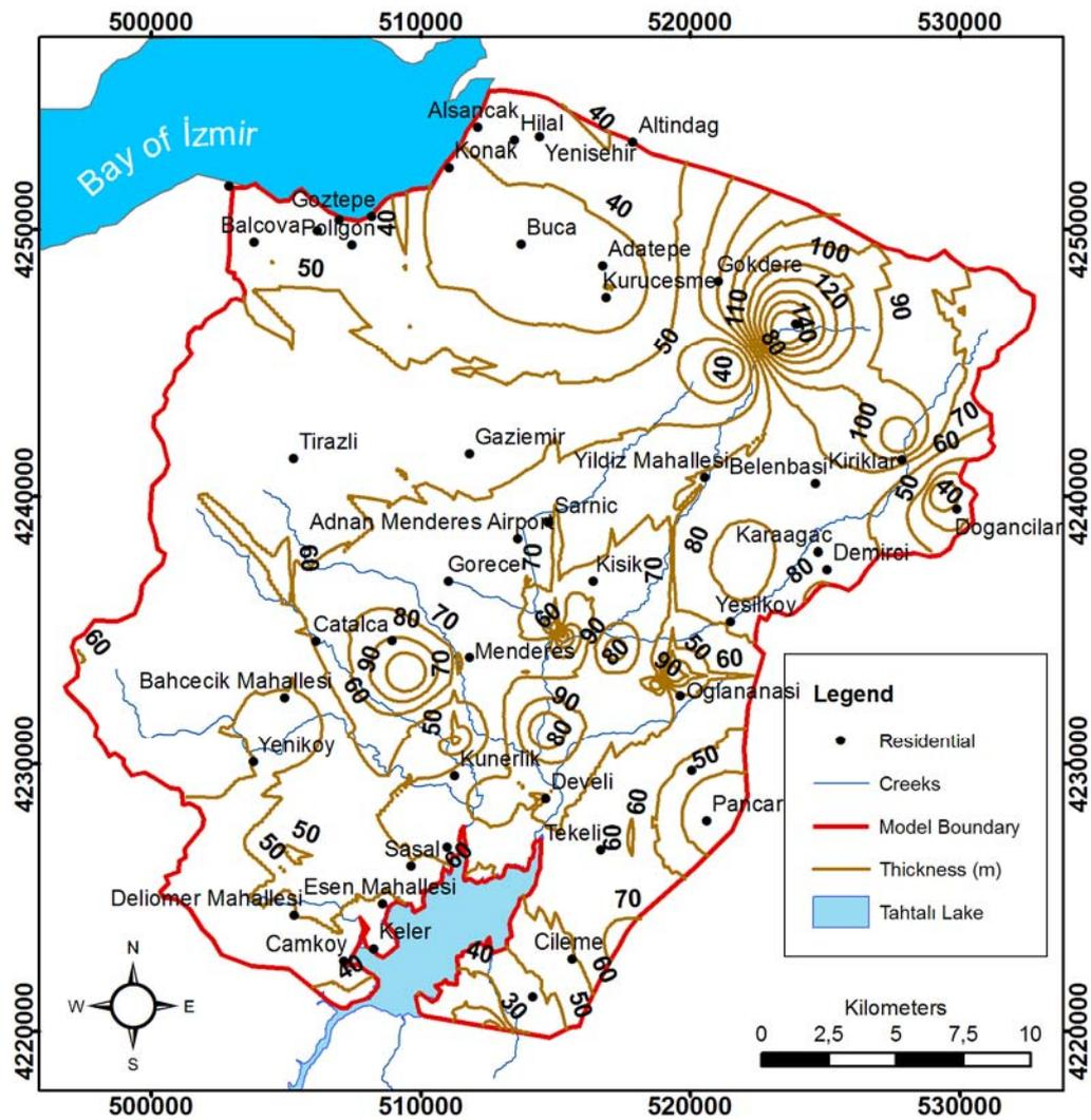
Figure 5.1 Isopach map showing the thickness of the model layer
