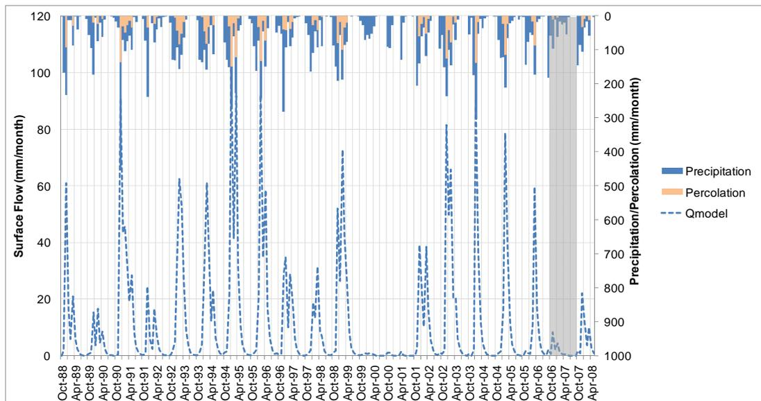
Figure 6.3 Results of the precipitation-runoff model; hydrographs for the predictive modeling period; the relevant period for the groundwater flow model is marked with the grey shaded area.
