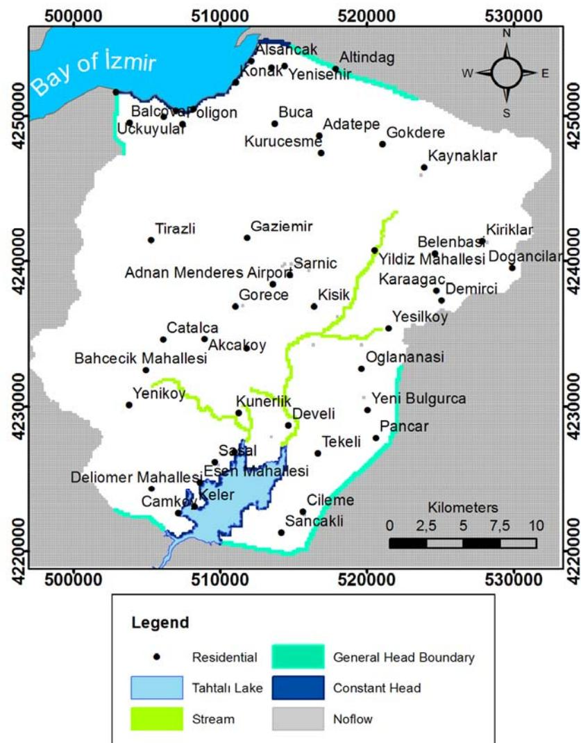
Figure 5.5 Boundary conditions used in the model
