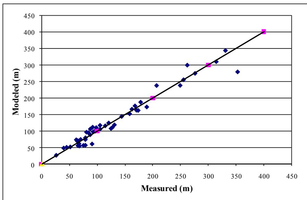
Figure 6.6 Comparison of modeled with measured head values for the calibrated model
