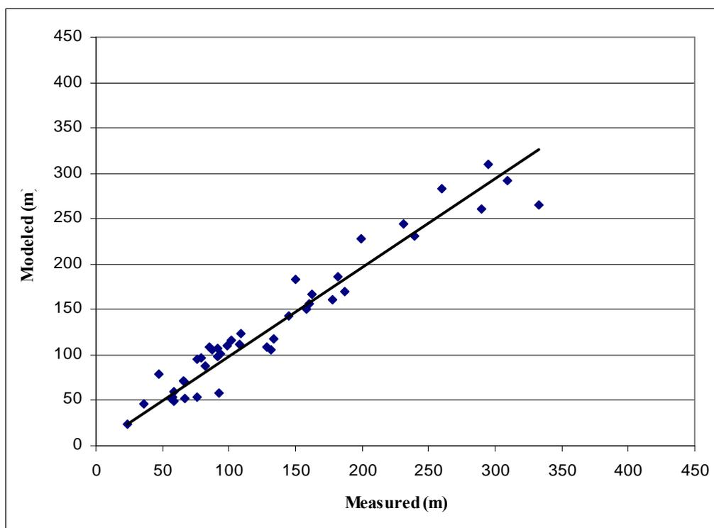
Figure 6.9 Comparison of modeled with measured head values for the verified model
