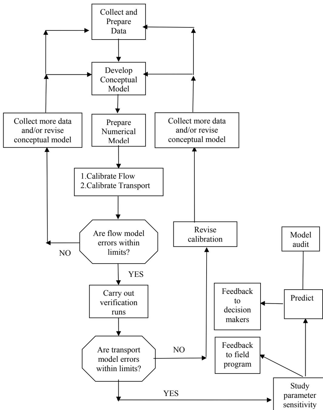
Figure 1.1 The groundwater modeling process
