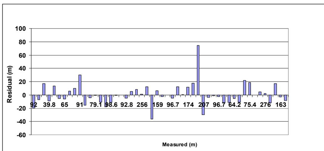
Figure 6.5 Comparison of residuals with observed values for the calibrated model
