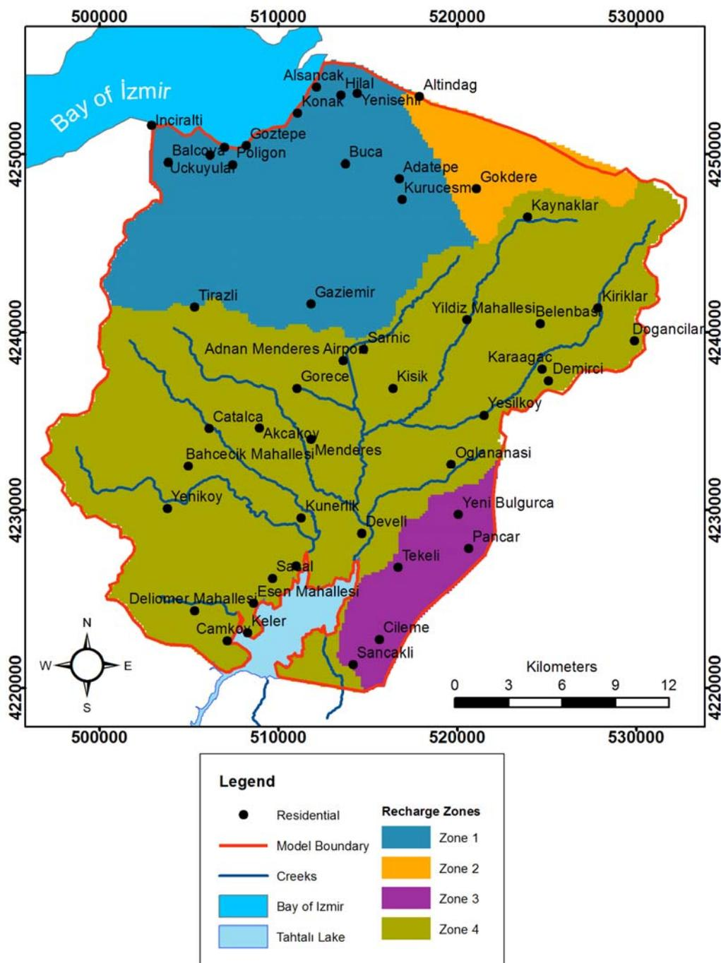
Figure 5.3 Recharge zones used in the model
