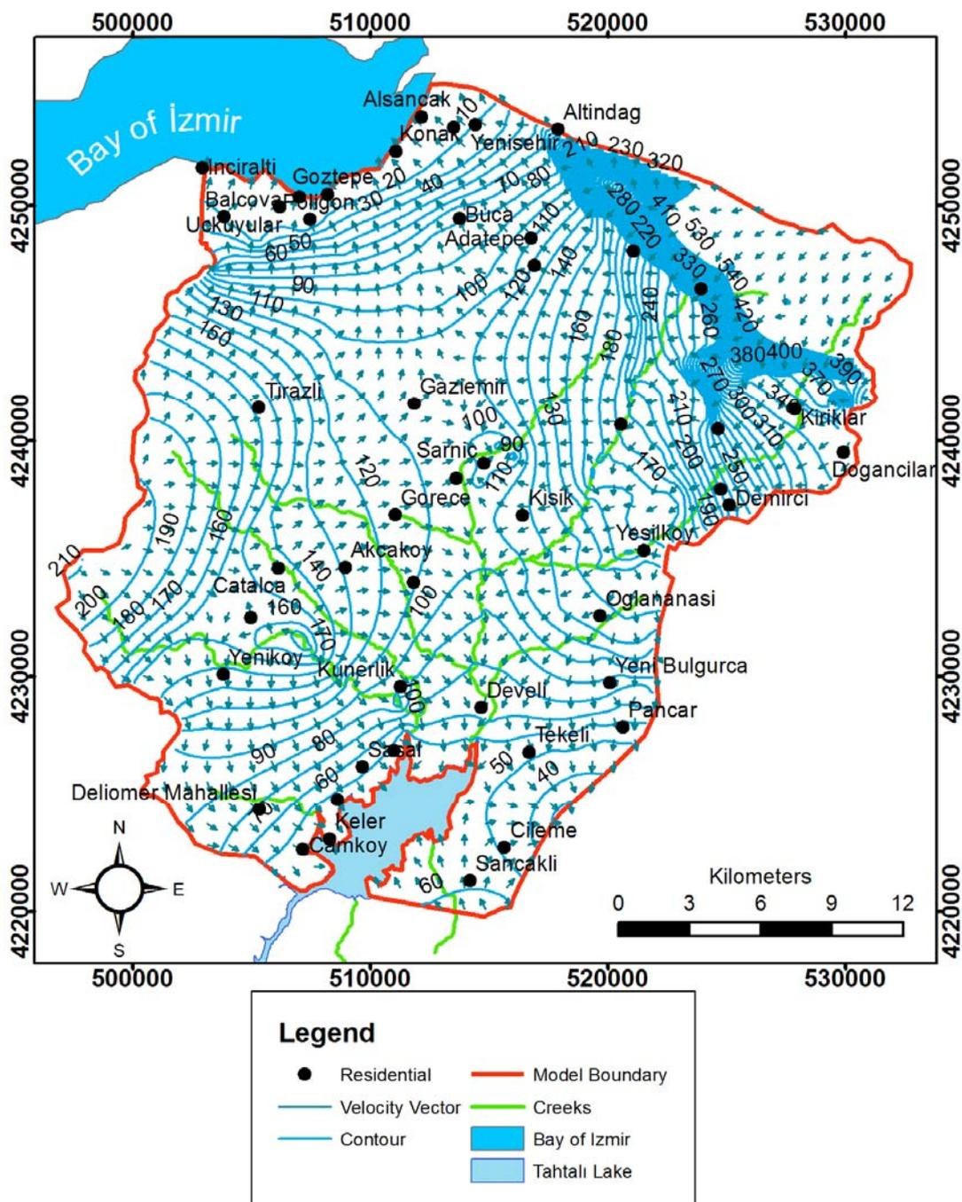
Figure 6.7 Groundwater flow modeling results: water table elevation contours and groundwater flow directions
