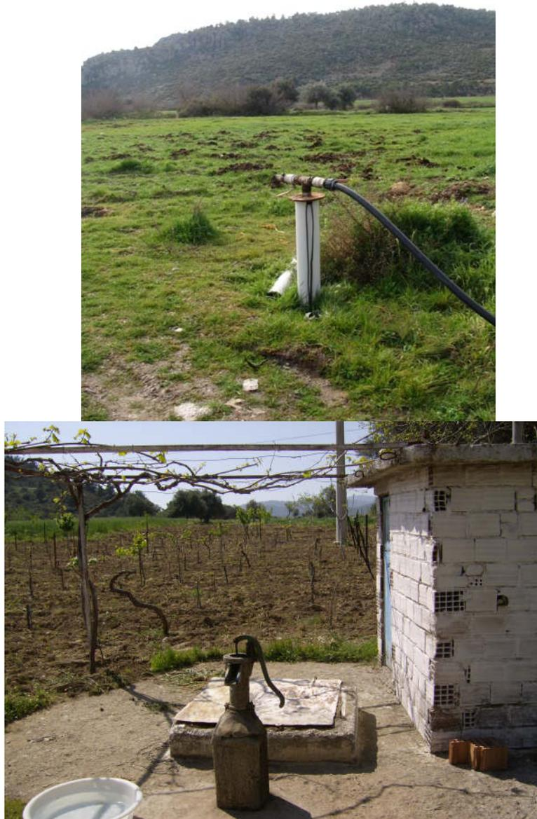
Figure 4.2 Different types of wells were selected for groundwater level measurements: deep irrigation well with an electrical submersible pump (above) and a shallow well with a lift pump (below)
