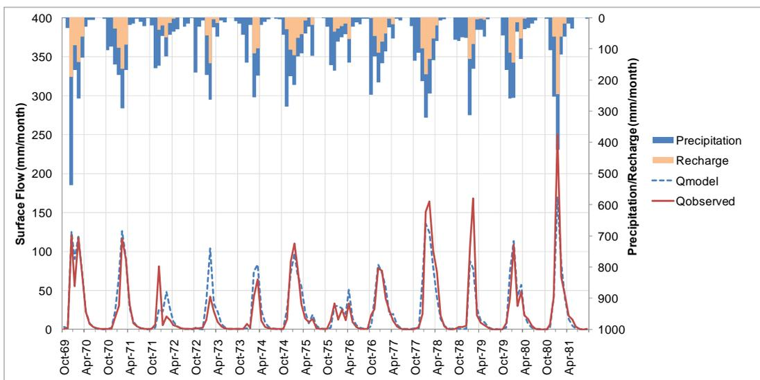
Figure 6.1 Results of the precipitation-runoff model; hydrographs for the verification period
