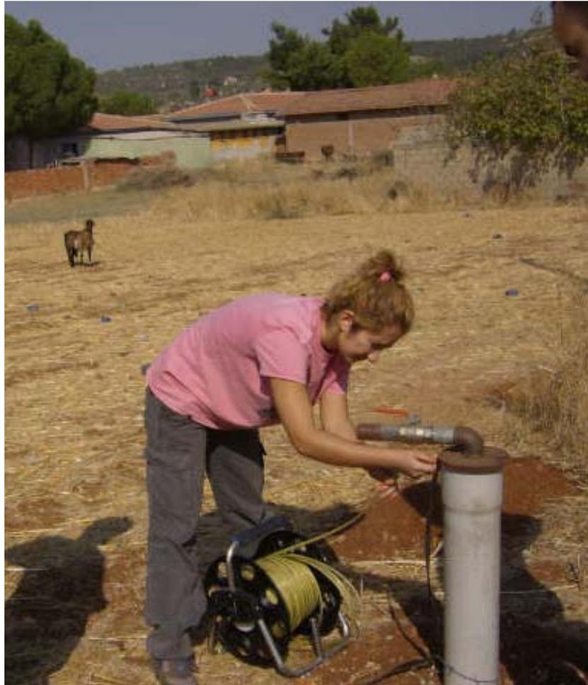
Figure 4.5 Measurement of the groundwater depth with a water level meter
