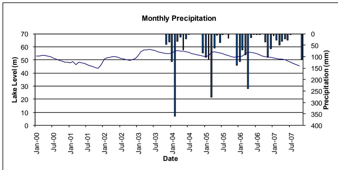
Figure 3.2 Monthly total water level records of the Tahtalı reservoir and monthly precipitation
