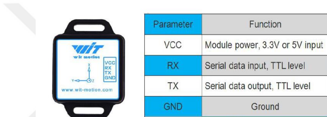
Figure 3.13 Pin description of MPU6050 sensor (Wit motion, n.d.)
