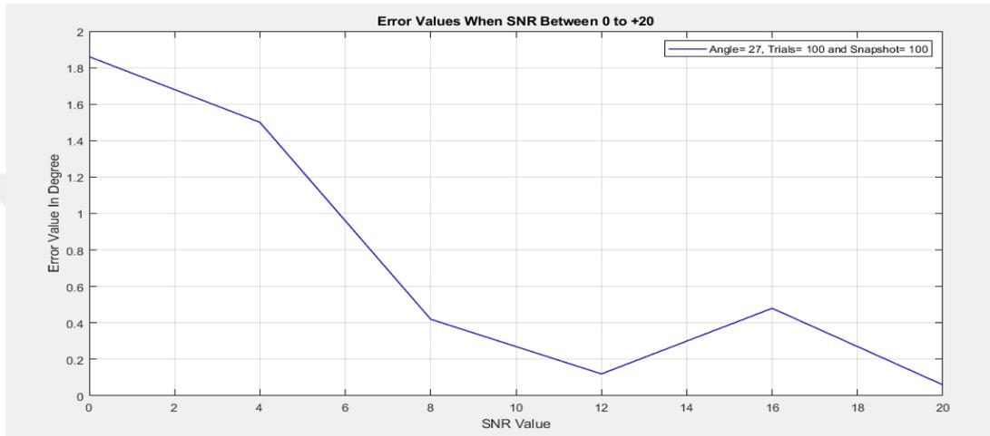
Figure 4.4 The Relation of the SNR and the error estimation of the ULSA structure
