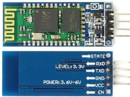
Figure 2.15 HC - 06 Bluetooth module (HC-06 Bluetooth Modul, 2016)
