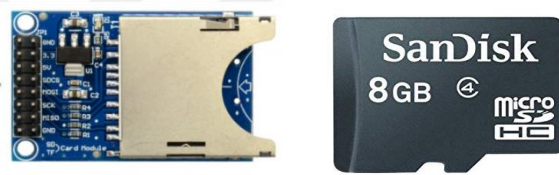
Figure 2.24 SD card module and SD card (Ada, 2019)
