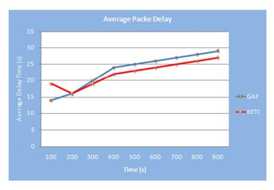
Figure 6.24 Average packet delay time in 900 seconds of network running with 100 nodes.
