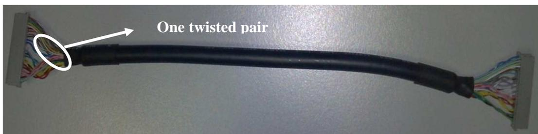
Figure 2.21 An LVDS cable connecting LVDS output of the TV mainboard to LVDS input of the picture grabbing card
