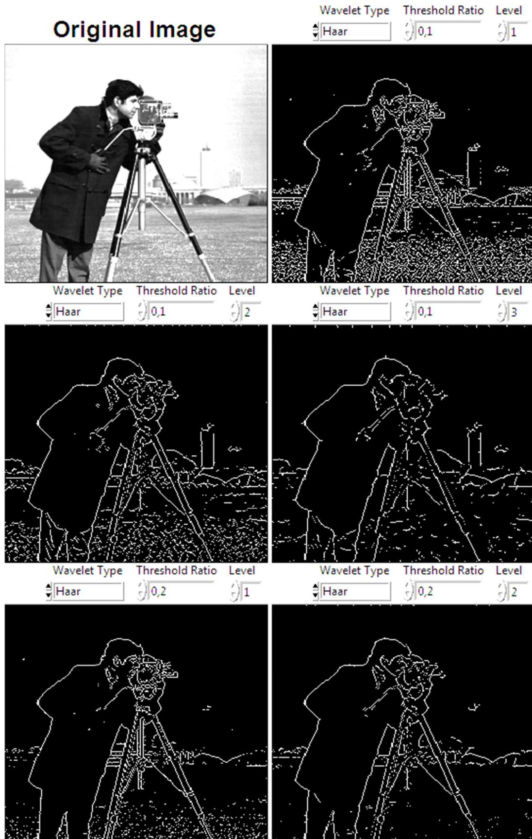
Figure 5.18 Wavelet based image edge detection with Haar wavelet
