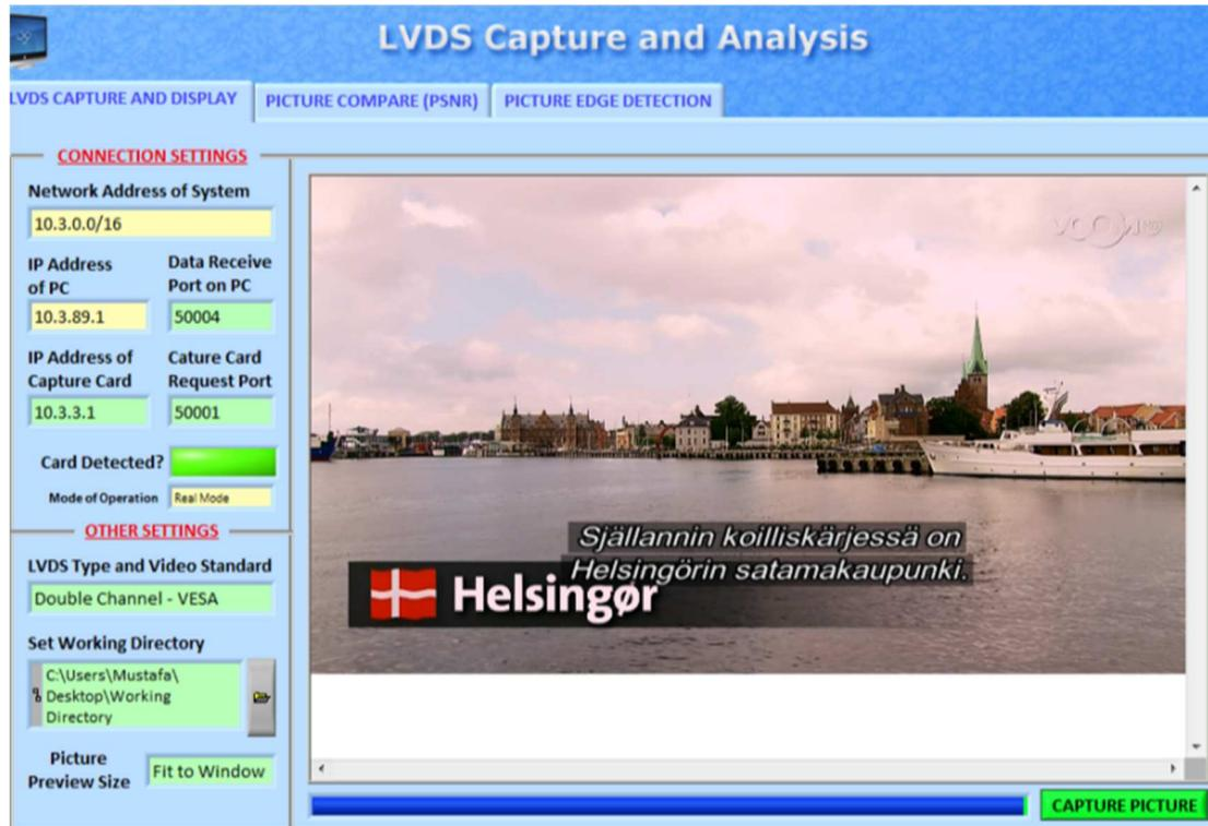
Figure 4.11 LVDS capture and display tab of the PC application software
