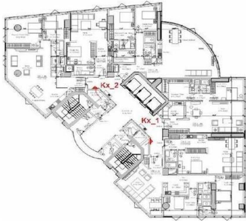
Figure 4.38.f Antenna installation positions: Floors between 7-23 (Kx\_1, Kx\_2; x=7 to 23)
