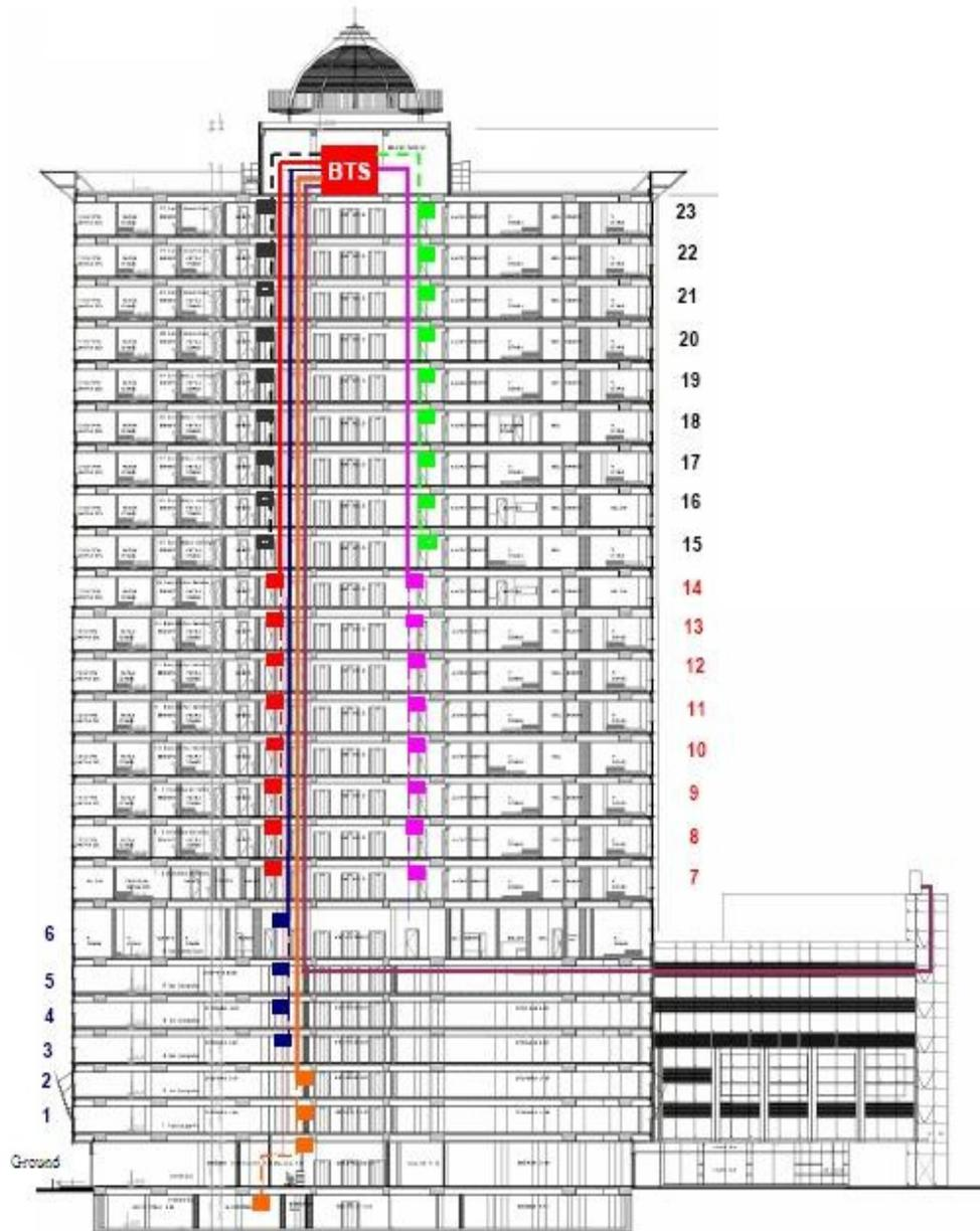
Figure 4.37 In-Building system design of a 23 floored plaza
