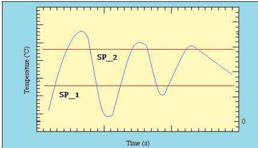
Figure 3.20 Hysteresis Characteristic Added On-Off Control Graphics
