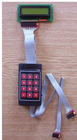
Figure 3.13 Digital display and keypad
