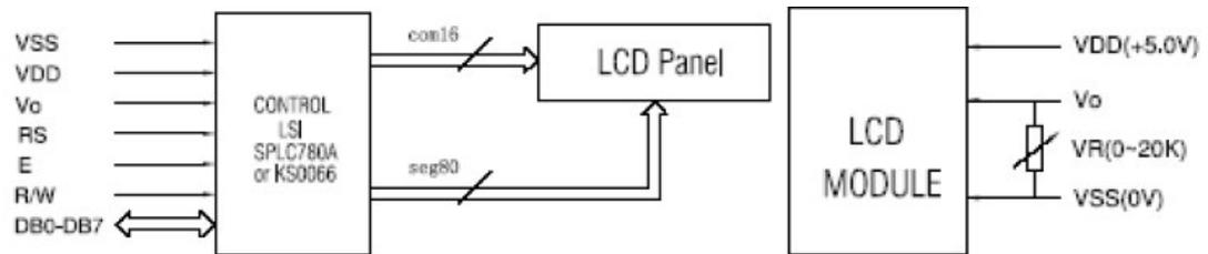
Figure 3.12 Input -output block diagram of LCD
