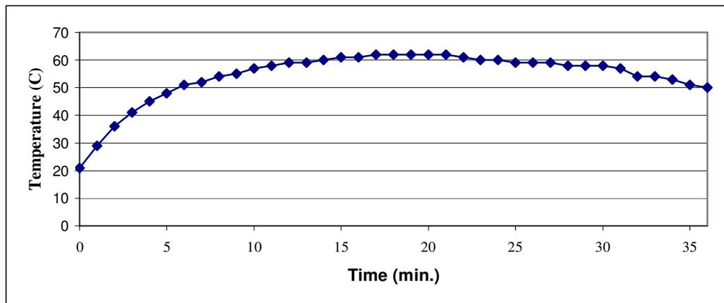
Figure 4.13 Temperature data of 3-ply, 2 panels trial
