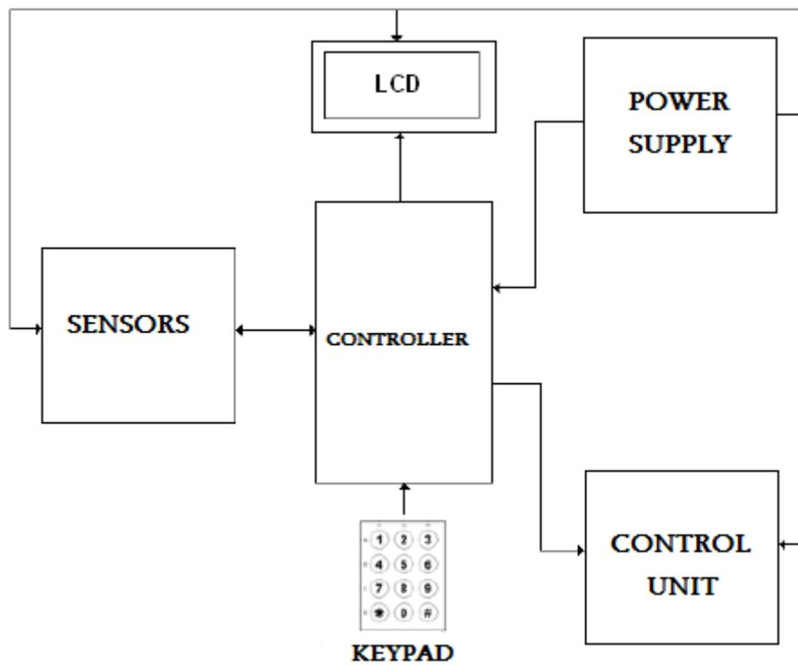
Figure 3.5 Block diagram of the heating control circuit
