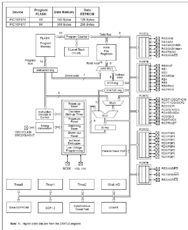
Figure 3.9 Block diagram of the PIC 16F877
