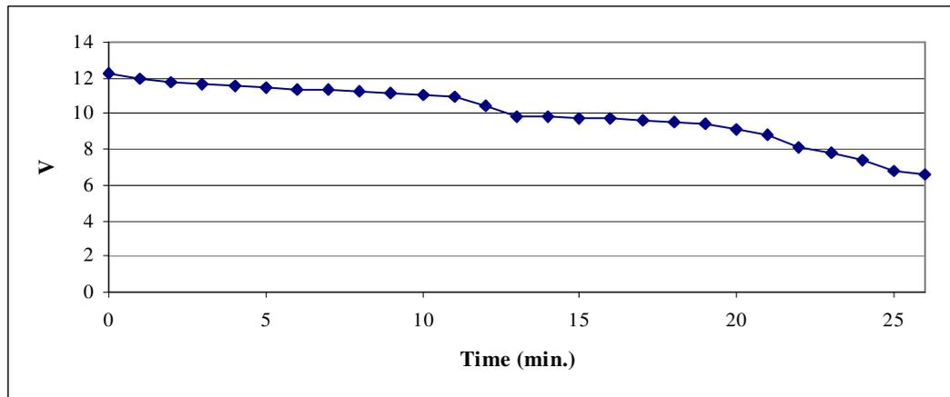
Figure 4.16 Voltage –time graphic of 4-ply, 2 panels trial
