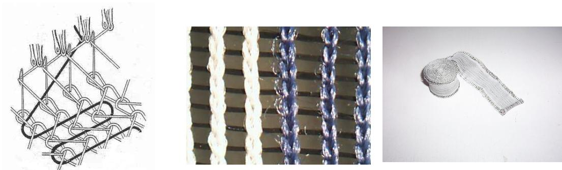
Figure 3.3 Formation of a heater panel by knitting with warp method
