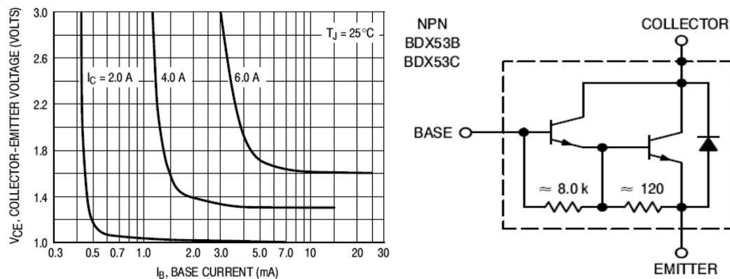
Figure 3.18 Collector-Emitter Saturation Voltage and internal schematic diagram
