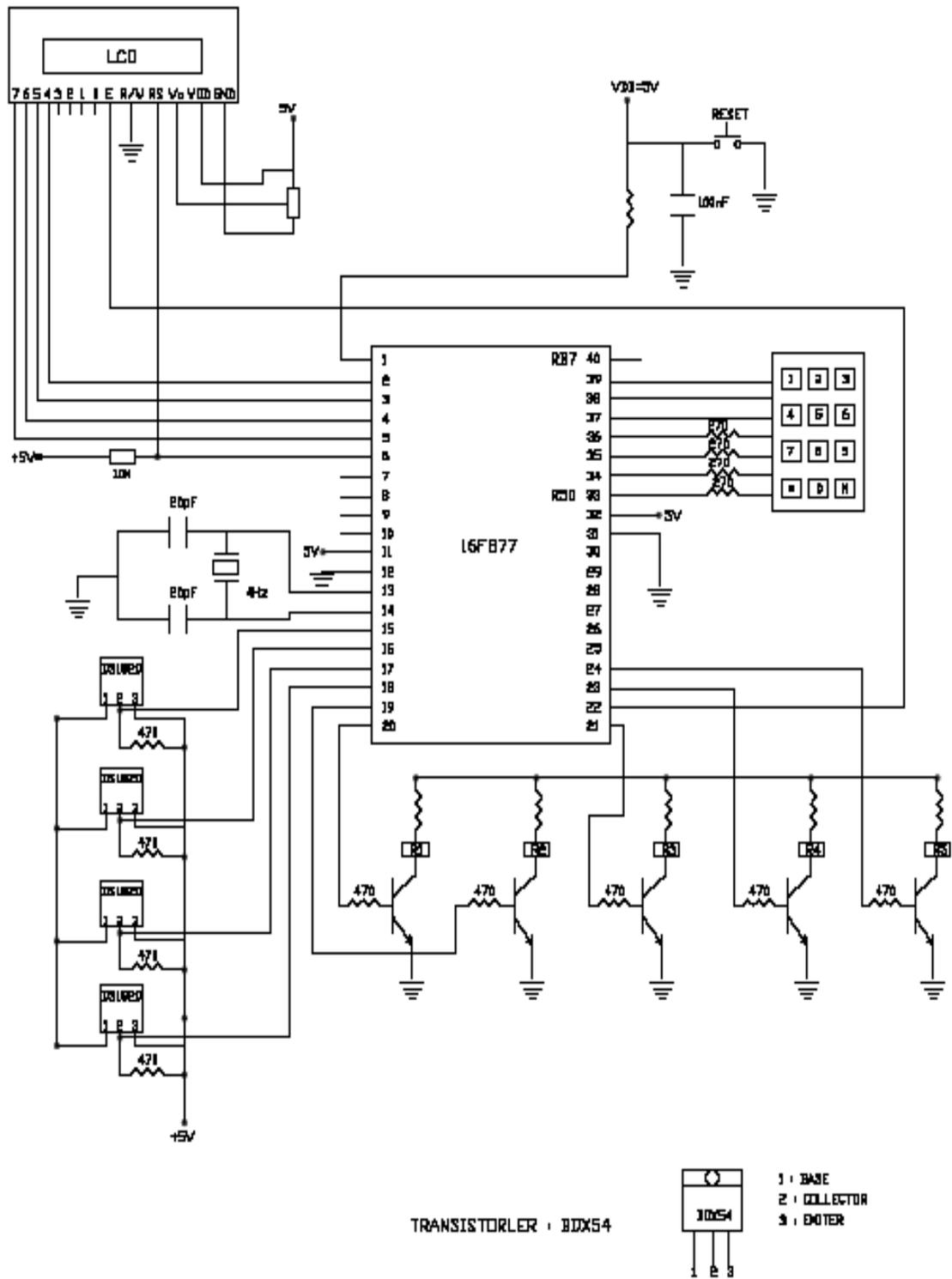
Figure 3.6 Circuit scheme for heating cloth prototype
