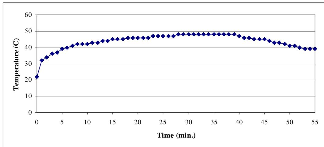
Figure 4.25 Temperature data of 1-ply, 4 panels trial
