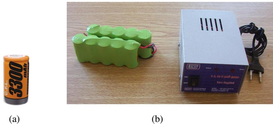
Figure 3.16 (a) Ni-MH battery (b) Ni-Mh battery group and charge device
