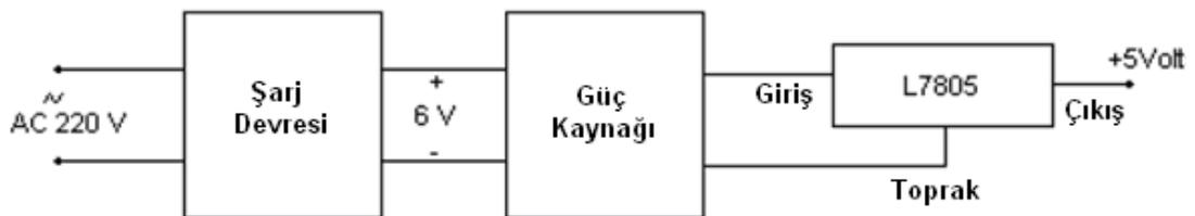
Figure 3.15 Power supply circuit
