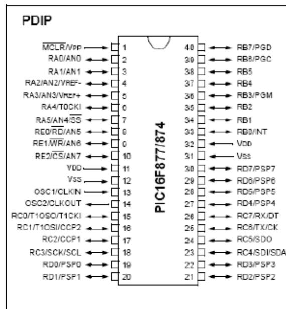
Figure 3.8 Pin diagram of the PIC 16F877
