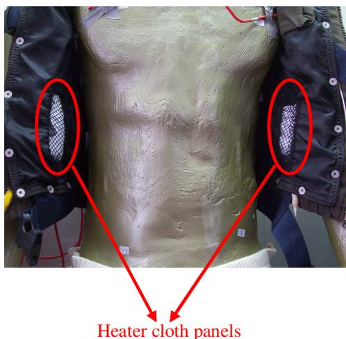
Figure 3.4 Location of the heater panels in clothes
