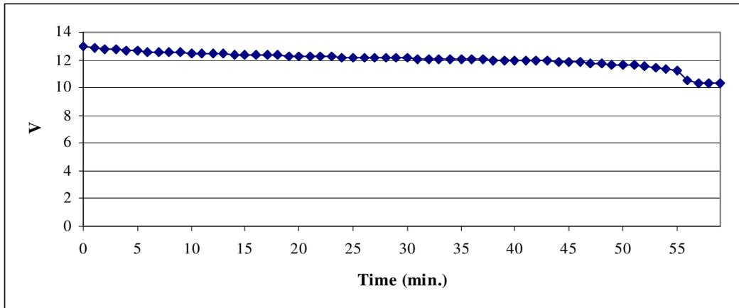
Figure 4.10 Voltage –time graphic of 1-ply, 2 panels trial
