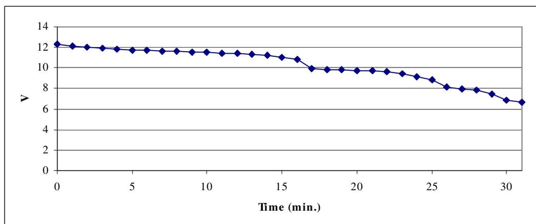
Figure 4.20 Voltage –time graphic of 2-ply, 3 panels trial
