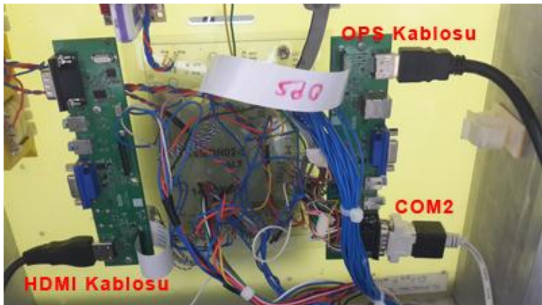
Figure 4.4 Monitor board test jig
