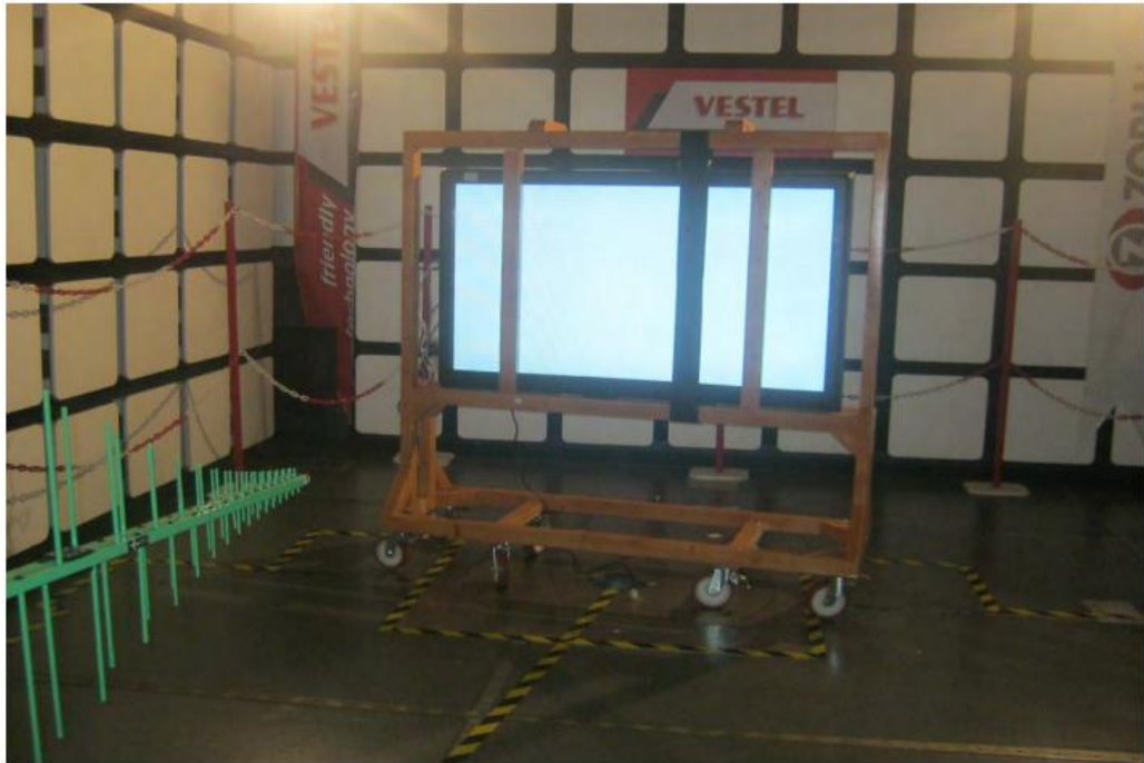
Figure 5.2 Radiated emission test at semi-anechoic chamber
