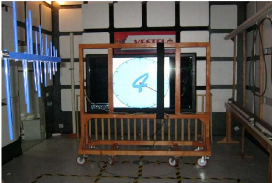
Figure 5.4 Radiated immunity tests at full-anechoic chamber
