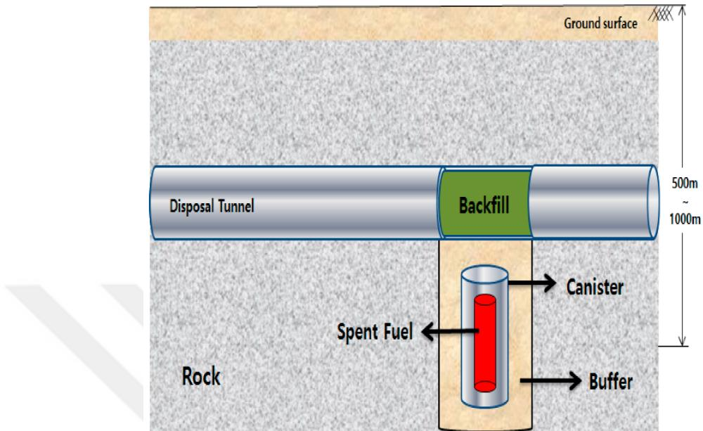
Figure 1.1 Conceptual nuclear waste repository model
