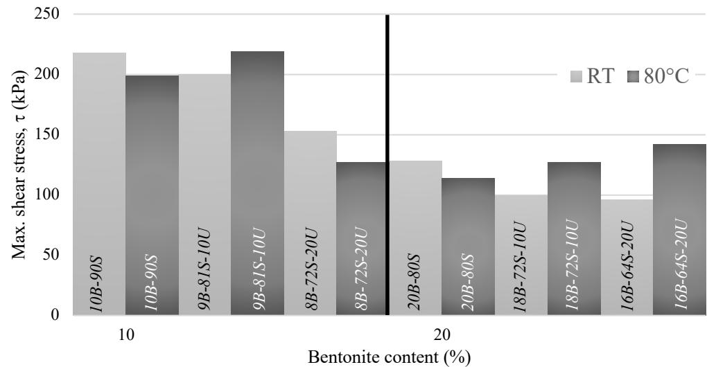
Figure 3.33 Maximum shear stress values of 10% and 20% sand-bentonite mixtures in the presence of ulexite at room temperature and at 80°C
