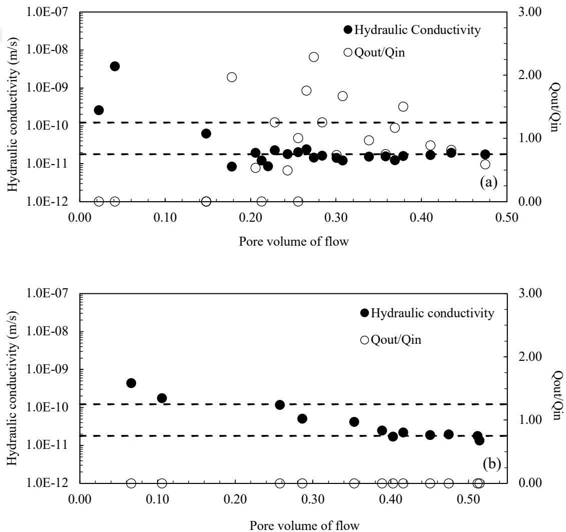
Figure 3.53 Hydraulic conductivity-PVF graphs of sand-bentonite mixtures at room temperature a)10B-90S b)20B-80S
