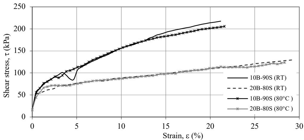
Figure 3.9 The shear stress-strain of 10B-90S and 20B-80S mixtures at room temperature and at 80°C
