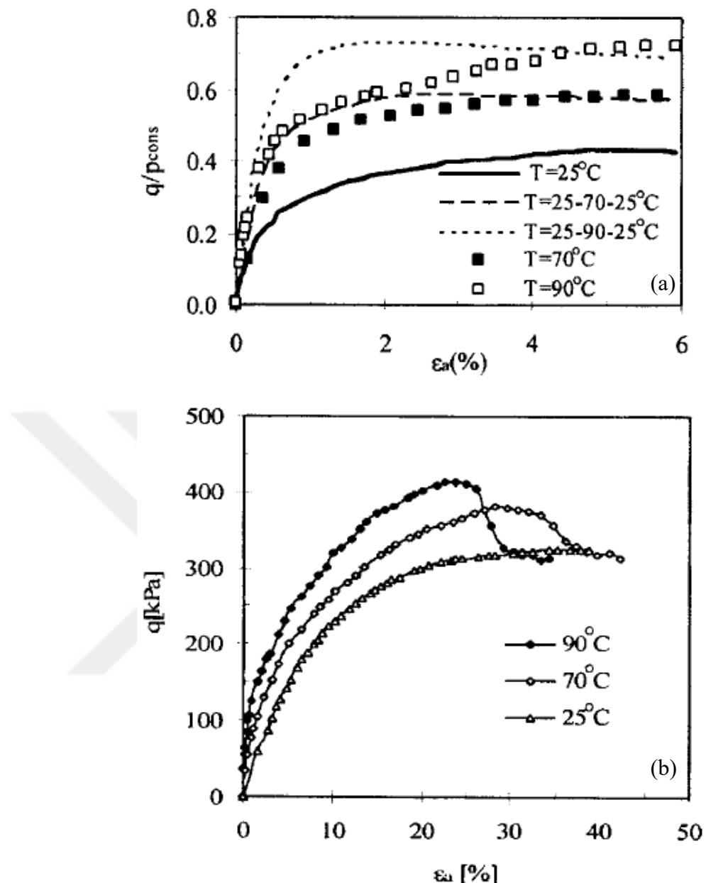
Figure 1.2 Triaxial compression tests on normally consolidated soft Bangkok clay a) Effect of temperature and temperature history on undrained test b) Drained test at different temperatures levels (Abuel-Naga, Bergado, & Ramana et al., 2006)
