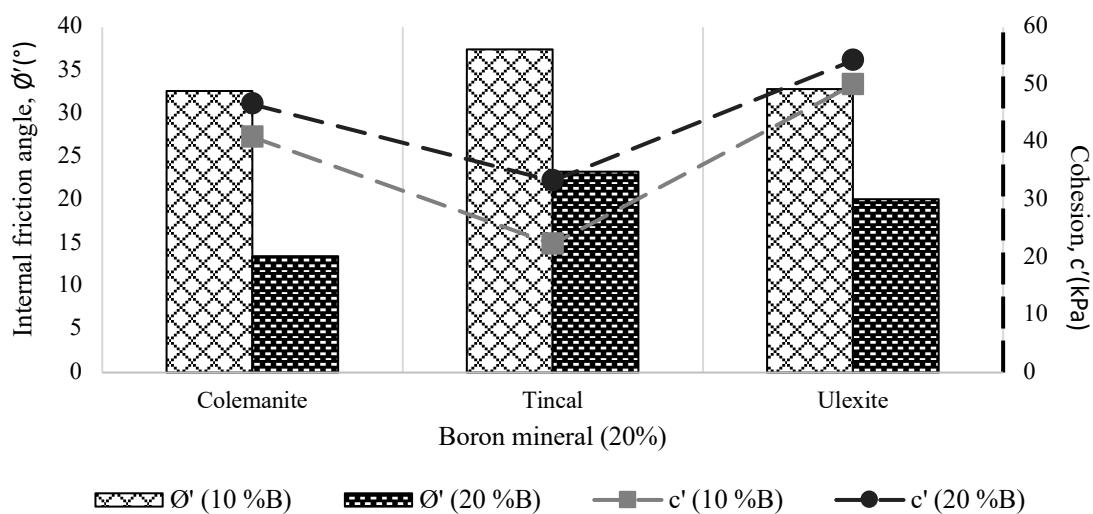
Figure 3.49 Internal friction angle and cohesion values according to boron mineral type for sand-bentonite mixtures in the presence of 20% boron at 80°C
