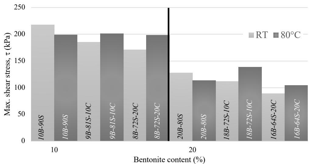
Figure 3.27 Maximum shear stress values of 10% and 20% sand-bentonite mixtures in the presence of colemanite at room temperature and 80°C
