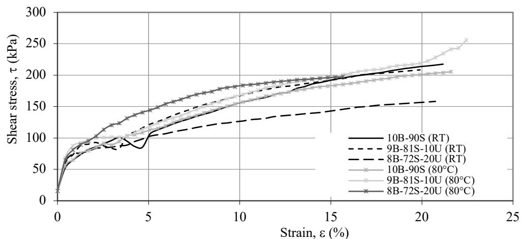
Figure 3.21 The shear stress-strain of 10% sand-bentonite mixtures in the presence of ulexite at room temperature and at 80°C
