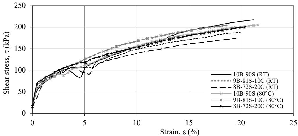
Figure 3.13 The shear stress-strain of 10% sand-bentonite mixtures in the presence of colemanite at room temperature and at 80°C
