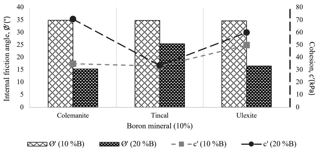
Figure 3.48 Internal friction angle and cohesion values according to boron mineral type for sand-bentonite mixtures in the presence of 10% boron at 80°C
