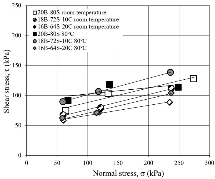
Figure 3.16 The shear failure envelopes of 20% sand-bentonite mixtures in the presence of colemanite at room temperature and at 80°C
