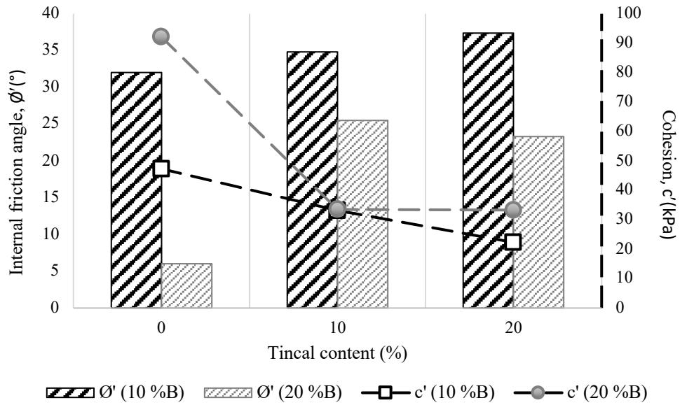
Figure 3.39 Internal friction angle and cohesion values depending on the tincal percentage of sand-bentonite mixtures at 80°C
