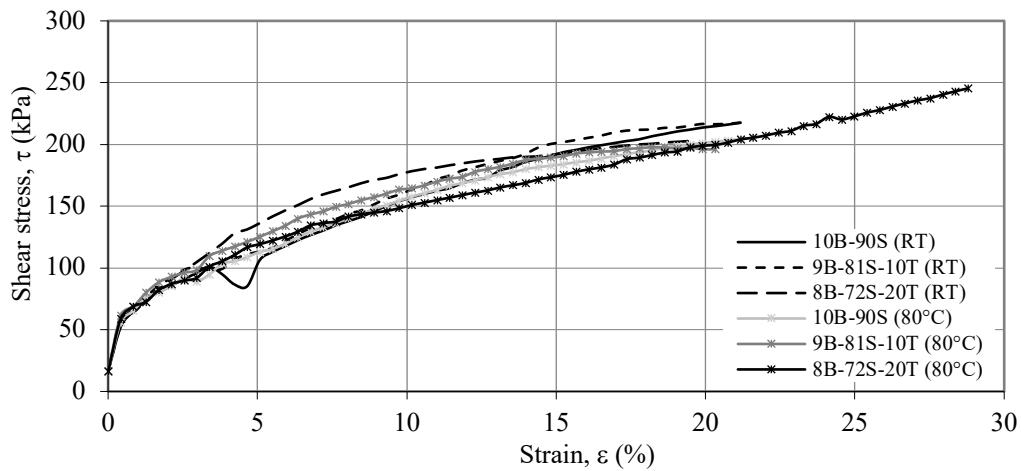
Figure 3.17 The shear stress-strain of 10% sand-bentonite mixtures in the presence of tincal at room temperature and at 80°C
