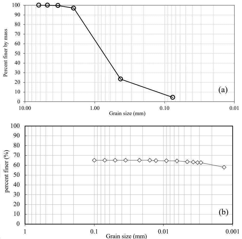
Figure 2.2 Grain size distribution of a) sand, b) bentonite
