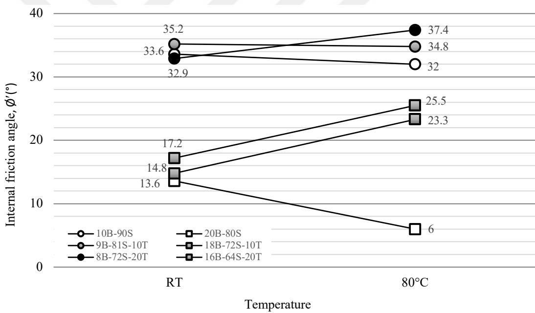
Figure 3.28 Internal friction angle values of 10% and 20% sand-bentonite mixtures in the presence of tincal at room temperature and at 80°C
