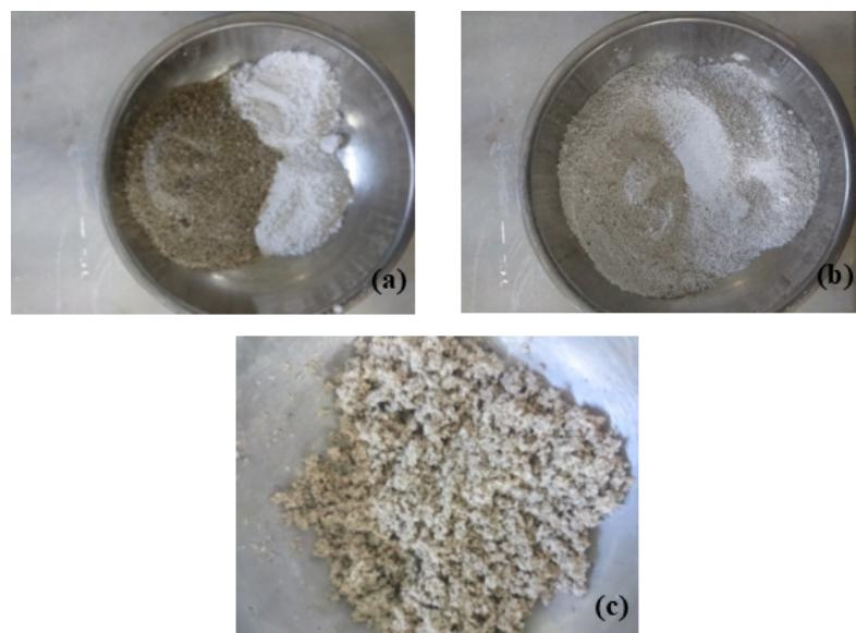
Figure 2.11 Preparation of the mixture for the shear test a) dry materials b) homogeneously mixed dry materials c) final mixture after water addition (Personal archive, 2019)
