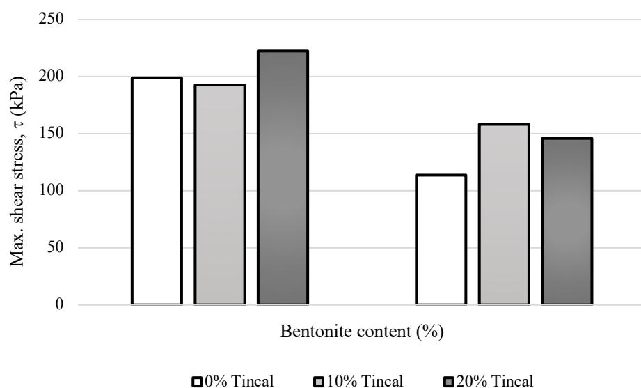
Figure 3.41 Maximum shear stress values depending on the tincal percentage of sand-bentonite mixtures at 80°C
