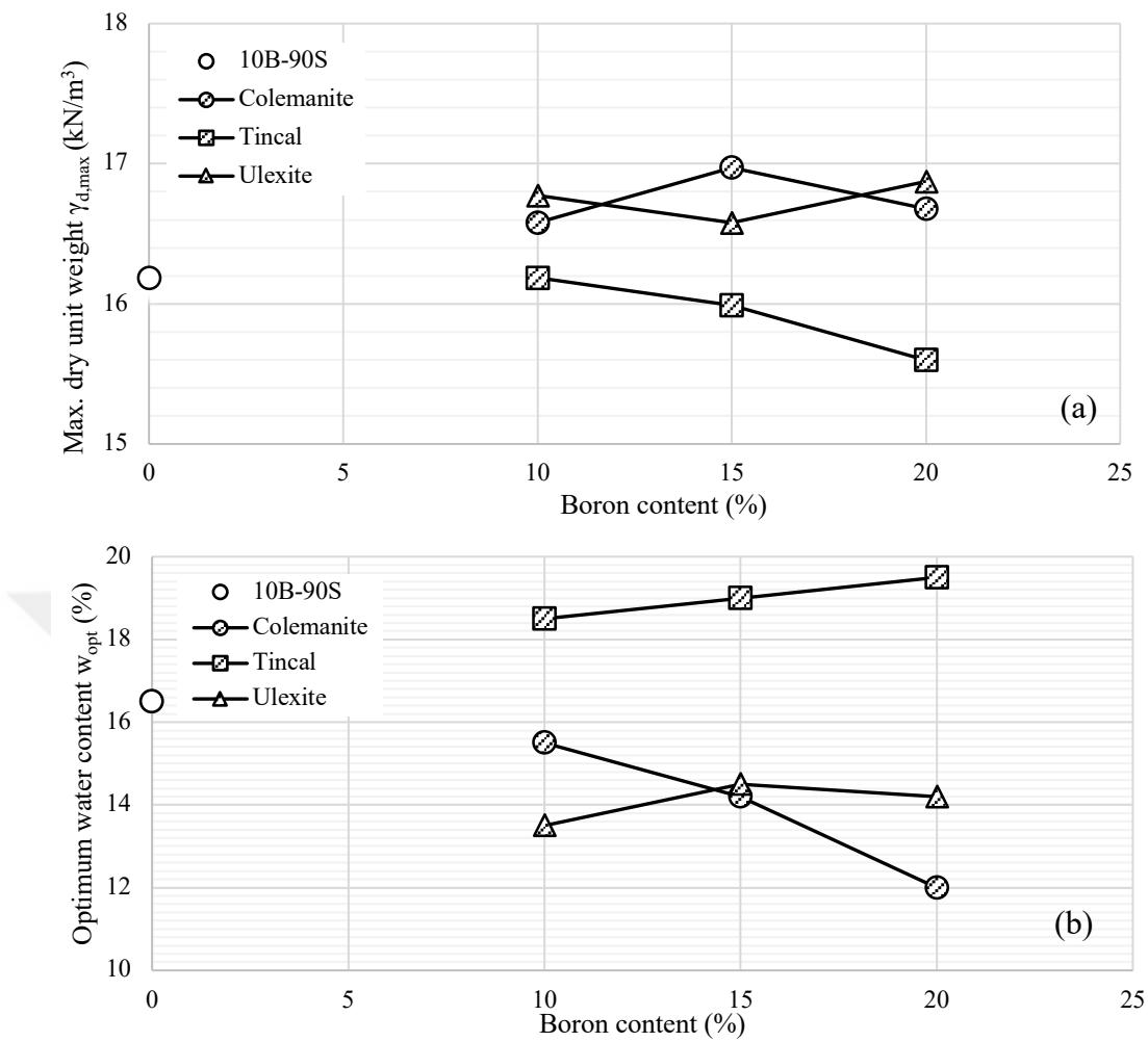
Figure 3.5 Compaction parameters a) max. dry unit weight b) optimum water content of 10% sand-bentonite mixtures in the presence of boron minerals
