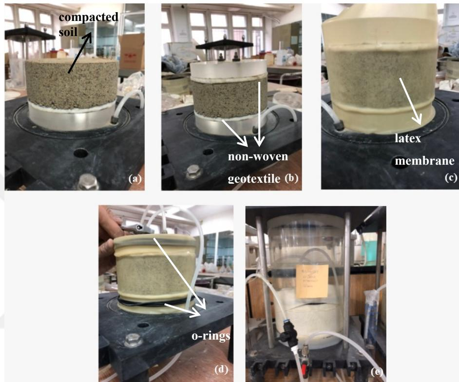
Figure 2.17 Preparation for hydraulic conductivity test a) Placement of the soil to the permeameter b) geotextiles placed on the top and bottom of the soil c) fitting latex membrane d) fitting of o-rings e) the permeameter after filling with water (Personal archive, 2018)
