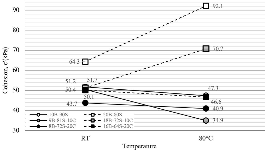
Figure 3.26 Cohesion values of 10% and 20% sand-bentonite mixtures in the presence of colemanite at room temperature and at 80°C
