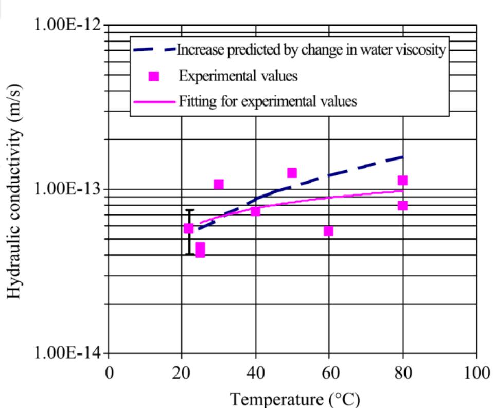
Figure 1.4 Comparison of hydraulic conductivity values determined experimentally and those predicted from the change in water kinematic viscosity at different temperatures (Villar & Lloret, 2004)
