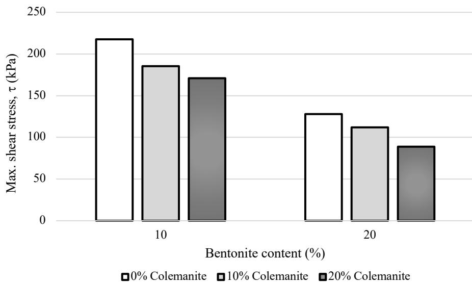
Figure 3.36 Maximum shear stress values depending on the colemanite percentage of sand-bentonite mixtures at room temperature
