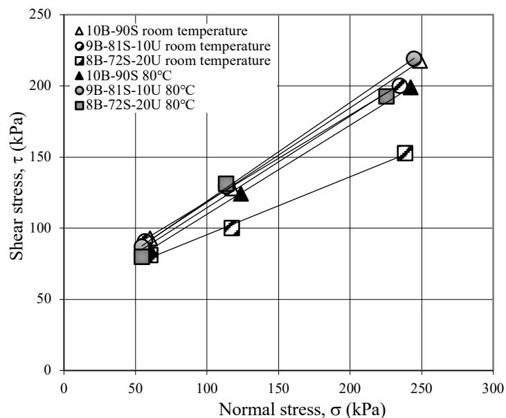
Figure 3.22 The shear failure envelopes of 10% sand-bentonite mixtures in the presence of ulexite at room temperature and at 80°C
