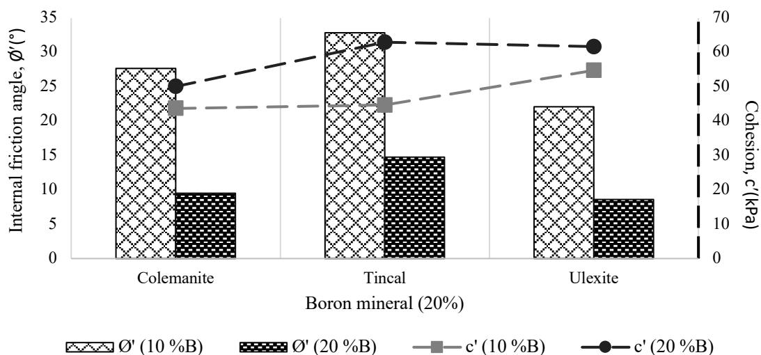
Figure 3.47 Internal friction angle and cohesion values according to boron mineral type for sand-bentonite mixtures in the presence of 20% boron at room temperature
