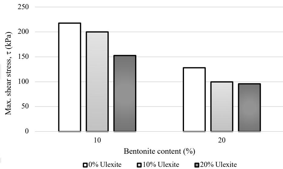
Figure 3.44 Maximum shear stress values depending on the ulexite percentage of sand-bentonite mixtures at room temperature
