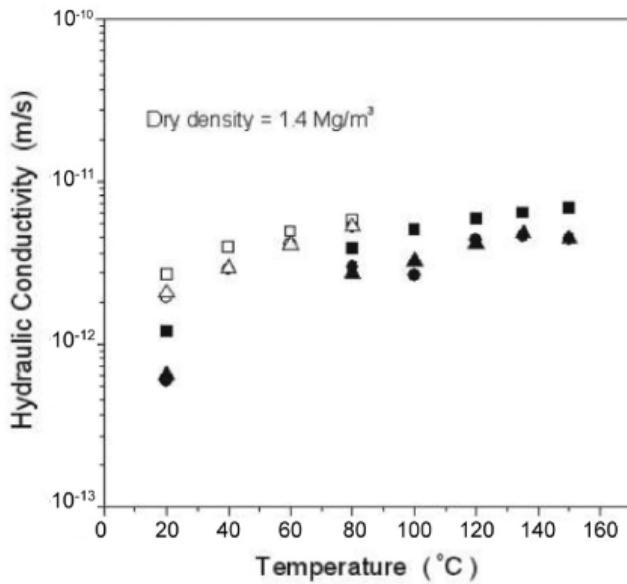
Figure 1.5 Hydraulic conductivity of compacted bentonite at different temperatures (Cho, Lee, & Kwon, 2011)
