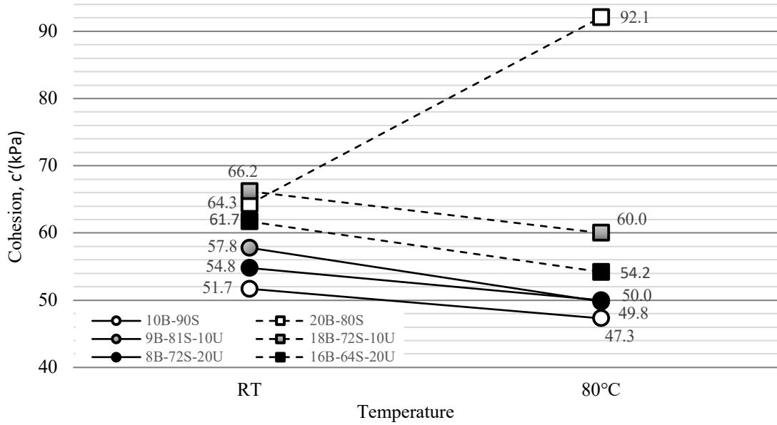
Figure 3.32 Cohesion values of 10% and 20% sand-bentonite mixtures in the presence of ulexite at room temperature and at 80°C
