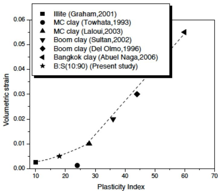
Figure 1.3 Volumetric strain with plasticity index of soil due to temperature change (Sinha & Kusakabe, 2008)
