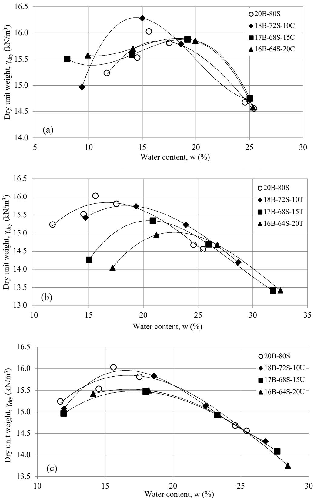
Figure 3.4 Compaction curves of 20% sand-bentonite mixtures in the presence of a) colemanite b) tincal c) ulexite
