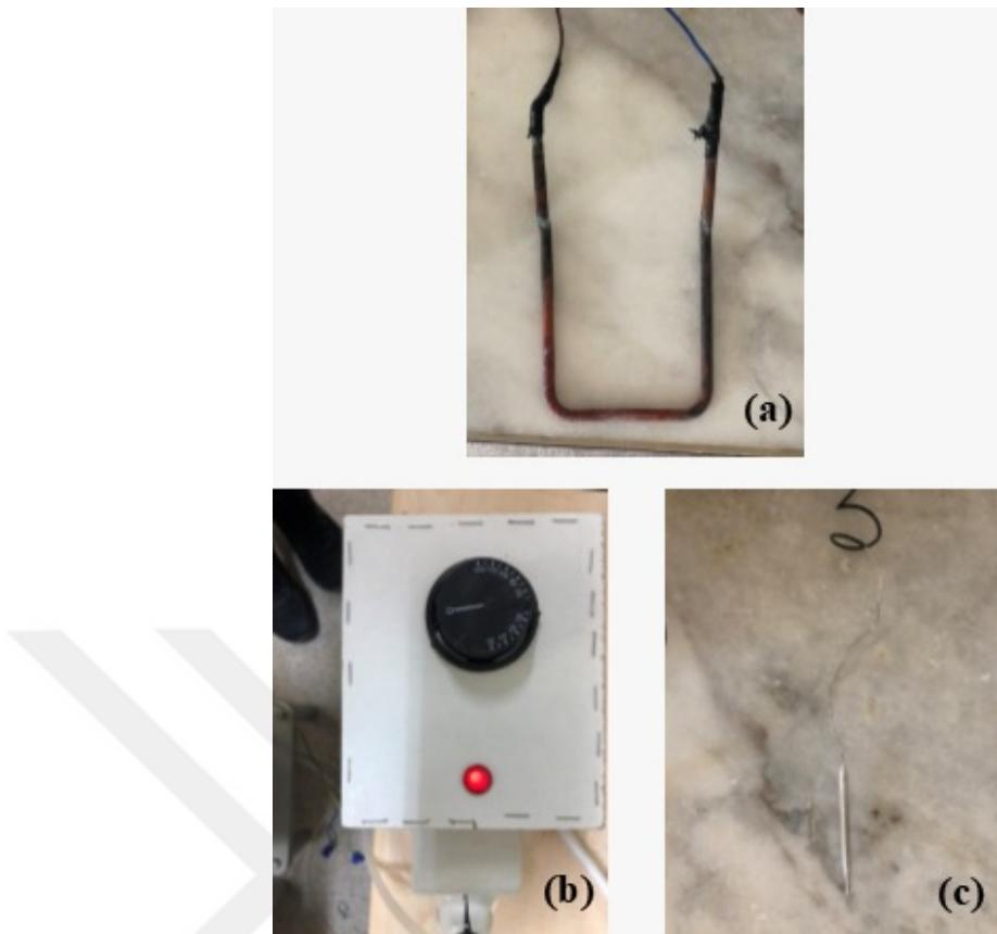
Figure 2.13 Heating tools for direct shear tests a) specially produced heat rod for the shear box b-c) thermostat for controlling water temperature (Personal archive, 2019)
