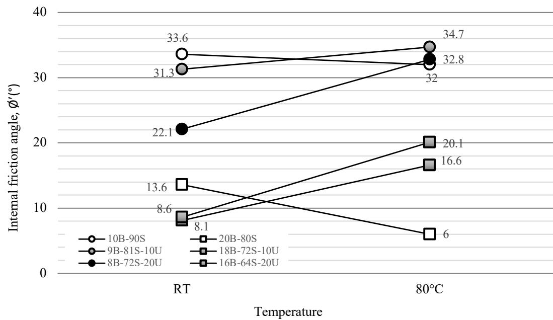
Figure 3.31 Internal friction angle values of 10% and 20% sand-bentonite mixtures in the presence of ulexite at room temperature and at 80°C
