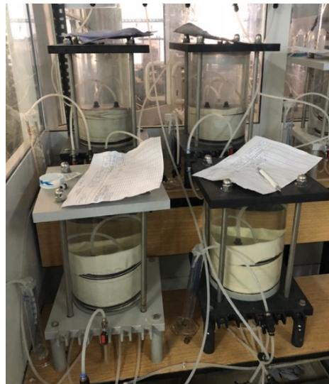
Figure 2.18 Hydraulic conductivity tests at room temperature (Personal archive, 2018)
