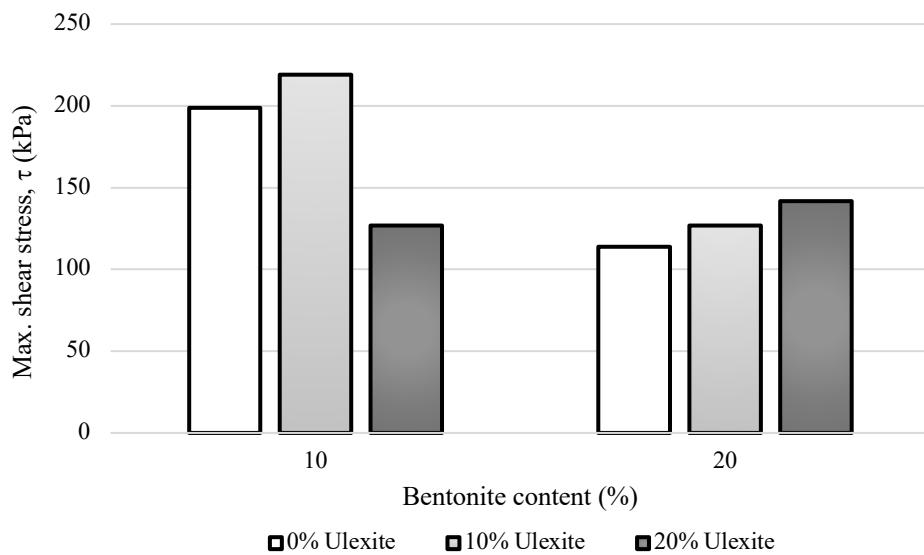
Figure 3.45 Maximum shear stress values depending on the ulexite percentage of sand-bentonite mixtures at 80°C
