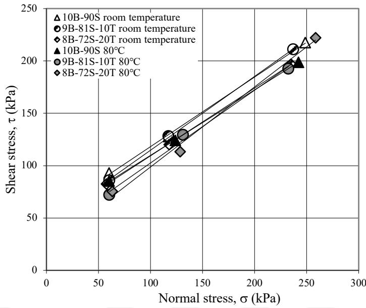
Figure 3.18 The shear failure envelopes of 10% sand-bentonite mixtures in the presence of tincal at room temperature and at 80°C
