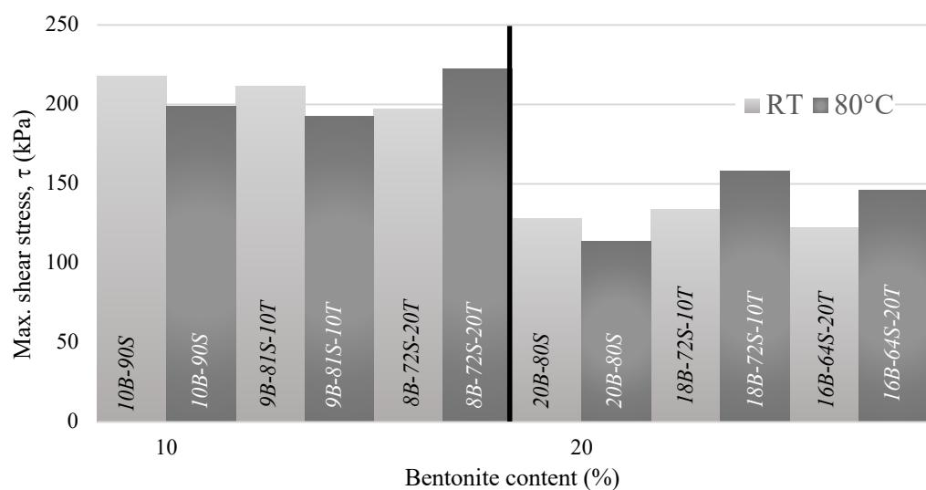
Figure 3.30 Maximum shear stress values of 10% and 20% sand-bentonite mixtures in the presence of tincal at room temperature and at 80°C
