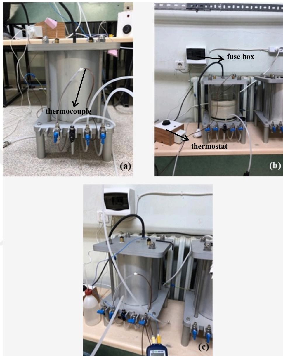
Figure 2.23 The hydraulic conductivity test system at 80°C a) passing the thermocouple through the valve b) thermostat system adjustment c) prevention with fuse box of electrical leakage (Personal archive, 2019)
