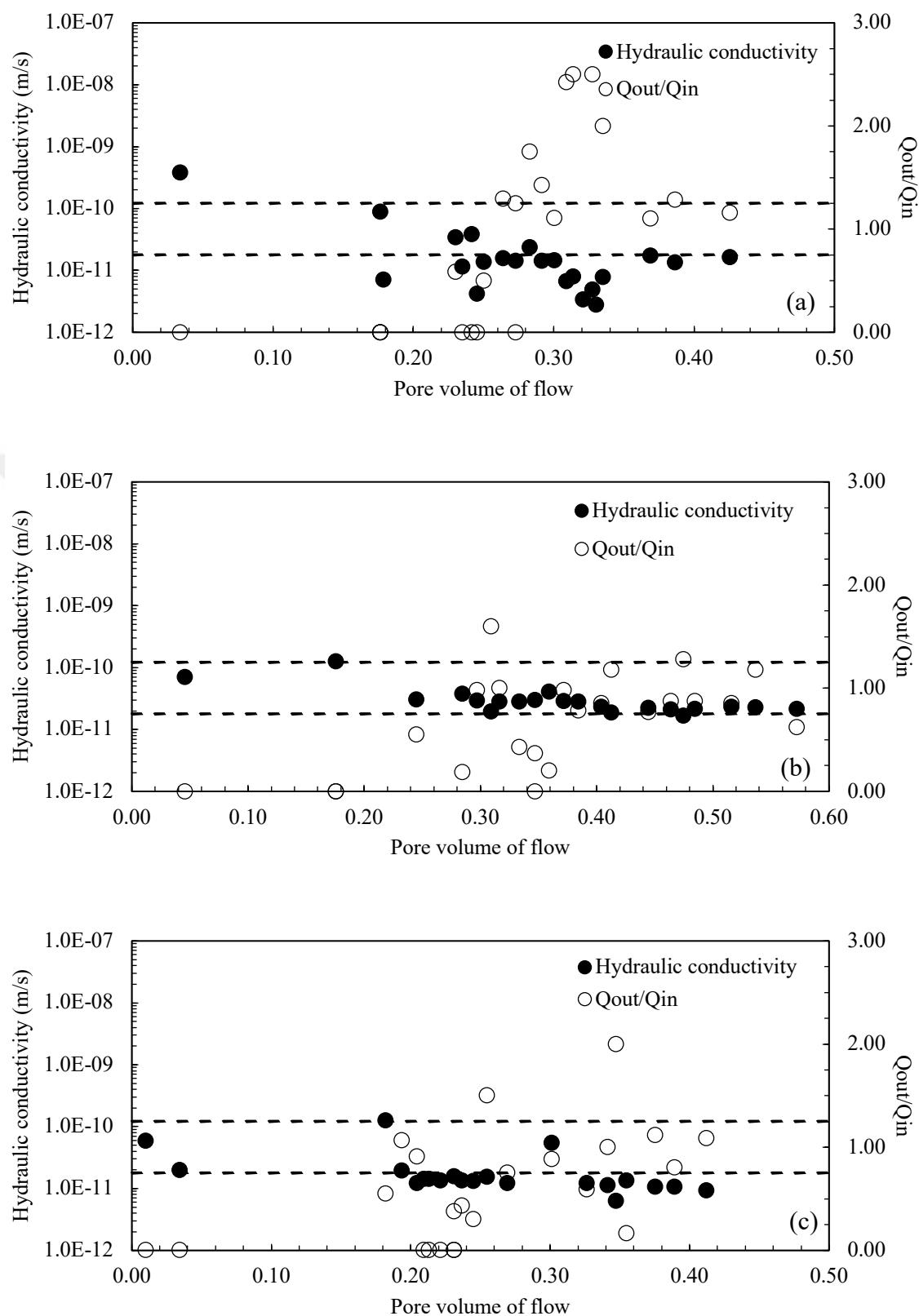
Figure 3.56 Hydraulic conductivity-PVF graphs of a)18B-72S-10T, b)17B-68S-15T, c)16B-64S-20T mixtures at room temperature
