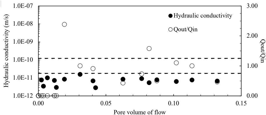
Figure 3.54 Hydraulic conductivity-PVF graphs of tincal at room temperature
