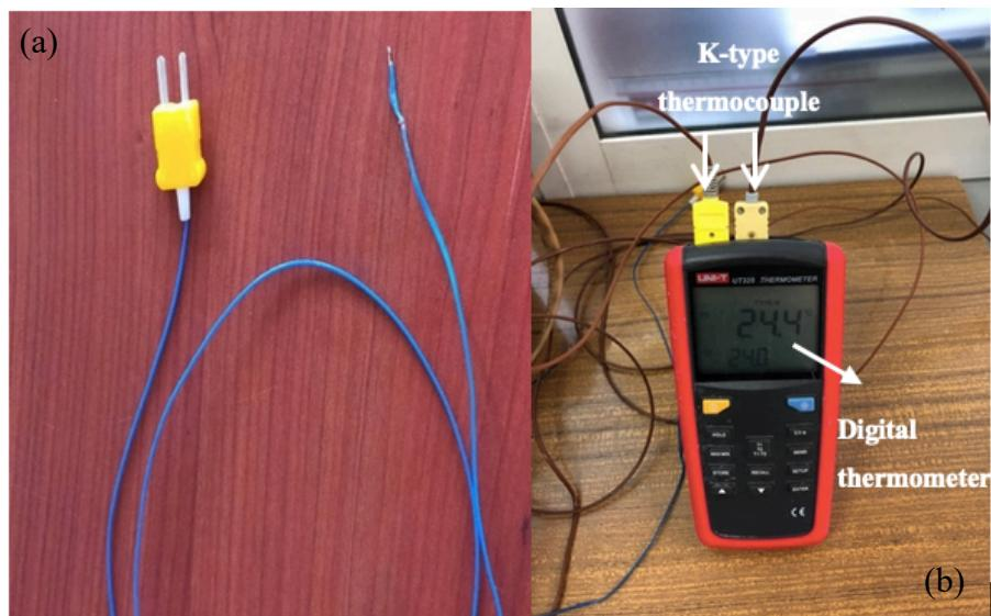
Figure 2.14 Tools for measuring and recording temperature during the tests under high temperature a) k-type thermocouple used in experiments b) digital thermometer (Personal archive, 2019)
