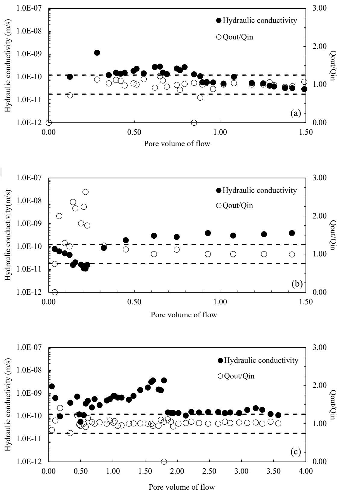
Figure 3.55 Hydraulic conductivity-PVF graphs of a) 9B-81S-10T, b) 8.5B-76.5S-15T, c) 8B-72S-20T mixtures at room temperature
