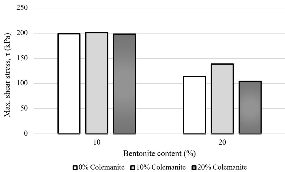
Figure 3.37 Maximum shear stress values depending on the colemanite percentage of sand-bentonite mixtures at 80°C
