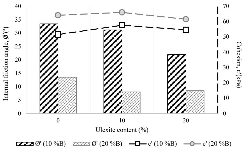
Figure 3.42 Internal friction angle and cohesion values depending on the ulexite percentage of sand-bentonite mixtures at room temperature
