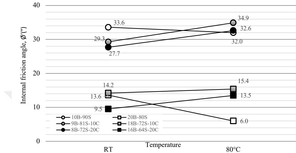
Figure 3.25 Internal friction angle values of 10% and 20% sand-bentonite mixtures in the presence of colemanite at room temperature and 80°C
