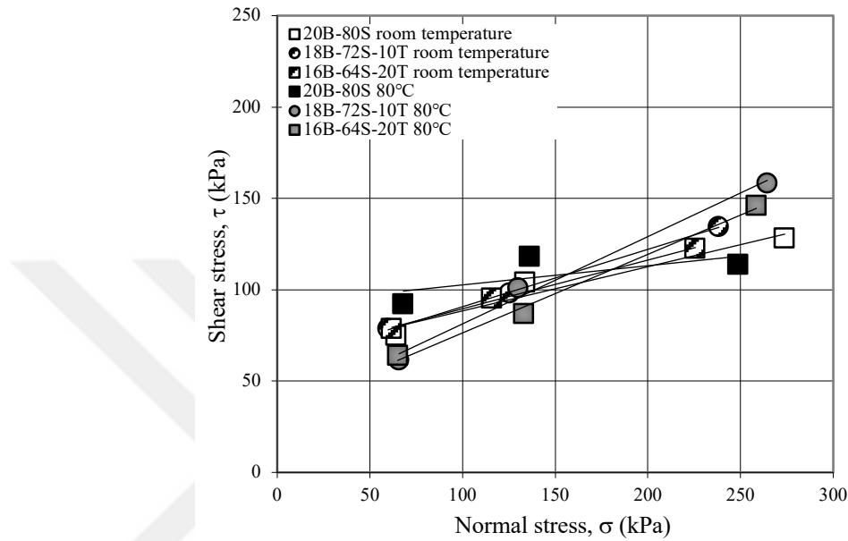
Figure 3.20 The shear failure envelopes of 20% sand-bentonite mixtures in the presence of tincal at room temperature and at 80°C
