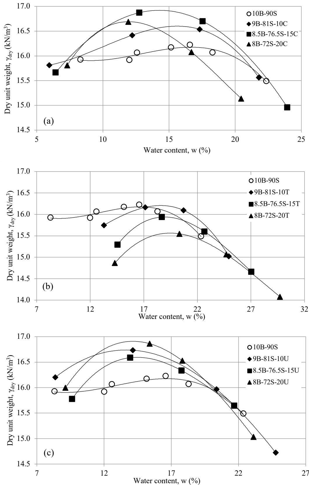
Figure 3.3 Compaction curves of 10% sand-bentonite mixtures in the presence of a) colemanite b) tincal c) ulexite
