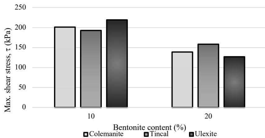
Figure 3.52 Maximum shear stress values according to boron mineral type for sand-bentonite mixtures in the presence of 10% boron at 80°C
