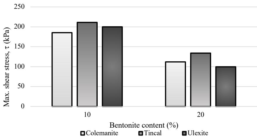
Figure 3.50 Maximum shear stress values according to boron mineral type for sand-bentonite mixtures in the presence of 10% boron at room temperature
