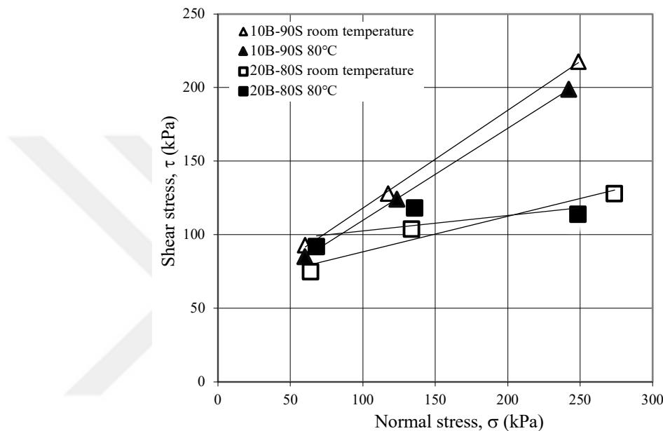
Figure 3.10 The shear failure envelopes of 10B-90S and 20B-80S at room temperature and at 80°C
