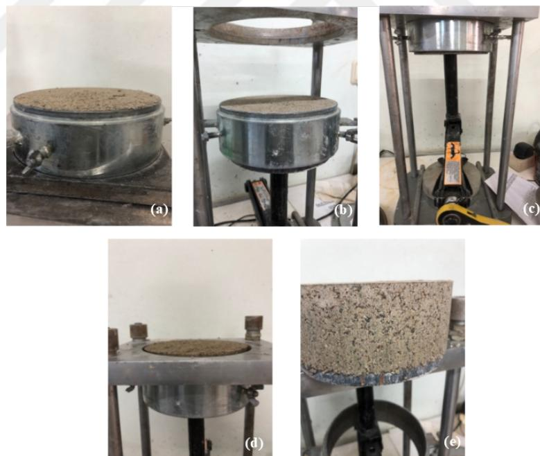
Figure 2.16 Sample preparation for hydraulic conductivity test a) compacted soil b-c-d) removed of compacted sample with hydraulic jack e) the sample removed from mold (Personal archive, 2018)
