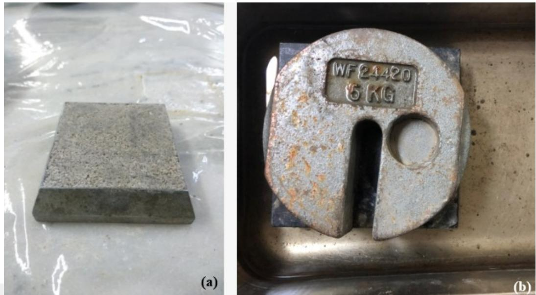
Figure 2.12 Sample preparation for shear test a) compacted sample in the mold b) submerged compacted sample (Personal archive, 2019)
