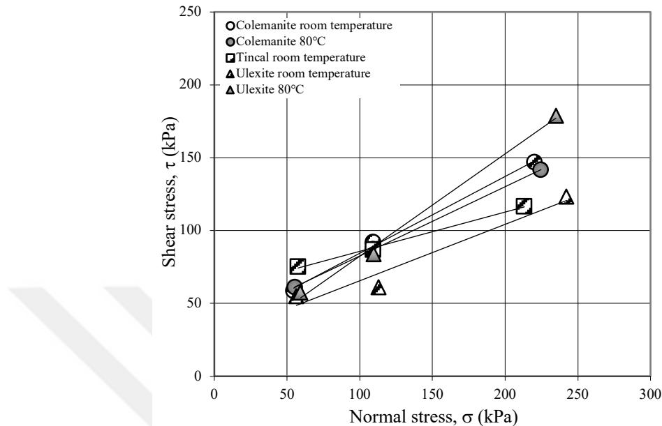
Figure 3.12 The shear failure envelopes of boron minerals at room temperature and at 80°C
