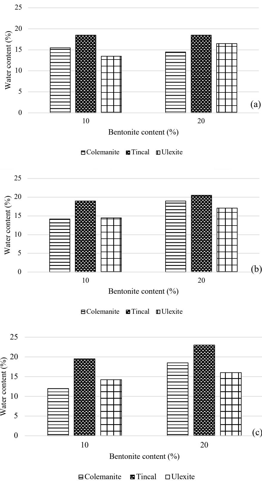
Figure 3.8 Optimum water content value according to boron mineral type a) 10% boron minerals b) 15% boron minerals c) 20% boron minerals
