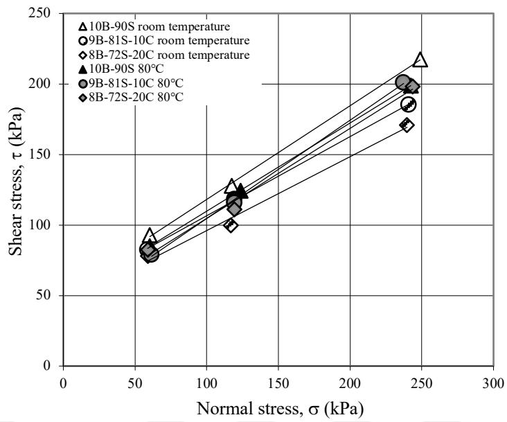
Figure 3.14 The shear failure envelopes of 10% sand-bentonite mixtures in the presence of colemanite at room temperature and at 80°C
