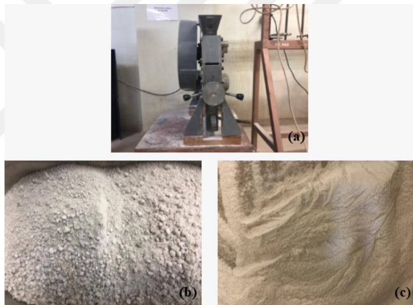
Figure 2.5 Preparation of tincal for tests a) jaw crusher to crush the tincal, b) crushed tincal, c) sieved tincal through No.40 (Personal archive, 2018)
