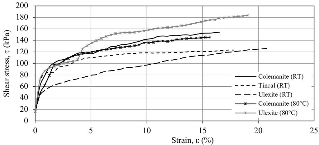
Figure 3.11 The shear stress-strain of boron minerals at room temperature and at 80°C
