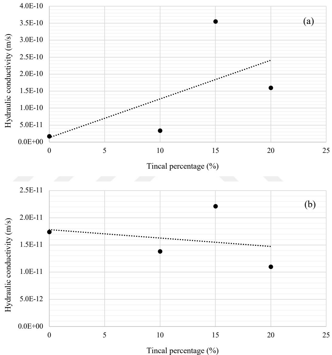
Figure 3.57 Hydraulic conductivity-tincal percentage graphs of mixtures a) 10% bentonite, b) 20% bentonite
