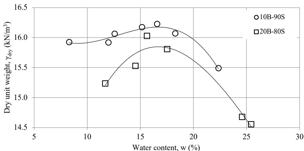
Figure 3.1 Compaction curves of sand-bentonite mixtures
