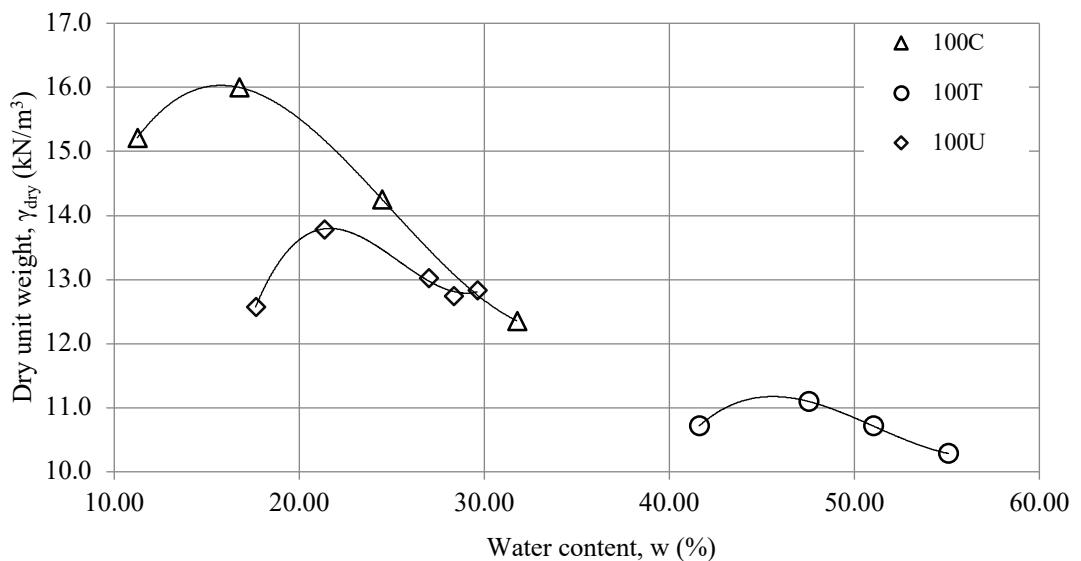
Figure 3.2 Compaction curves of boron minerals
