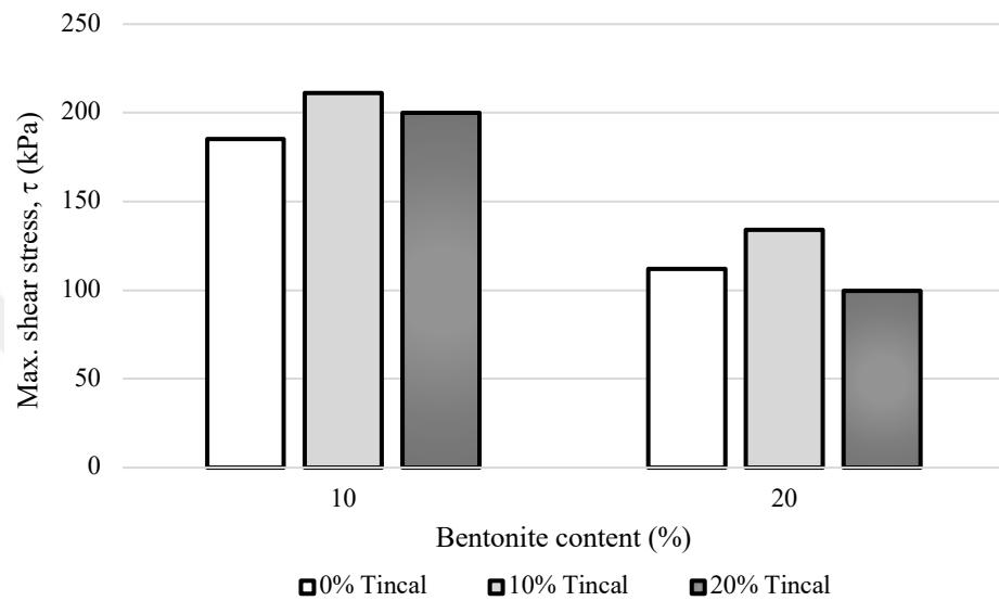
Figure 3.40 Maximum shear stress values depending on the tincal percentage of sand-bentonite mixtures at room temperature
