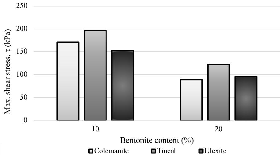
Figure 3.51 Maximum shear stress values according to boron mineral type for sand-bentonite mixtures in the presence of 20% boron at room temperature
