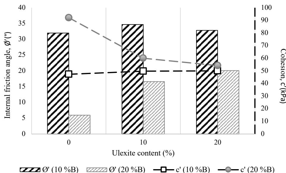
Figure 3.43 Internal friction angle and cohesion values depending on the ulexite percentage of sand-bentonite mixtures at 80°C
