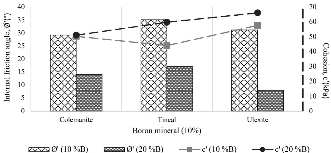
Figure 3.46 Internal friction angle and cohesion values according to boron mineral type for sand-bentonite mixtures in the presence of 10% boron at room temperature
