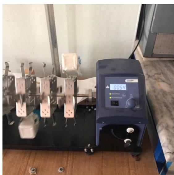
Figure 2.6 Shaking the plastic container on the shaker (Personal archive, 2019)
