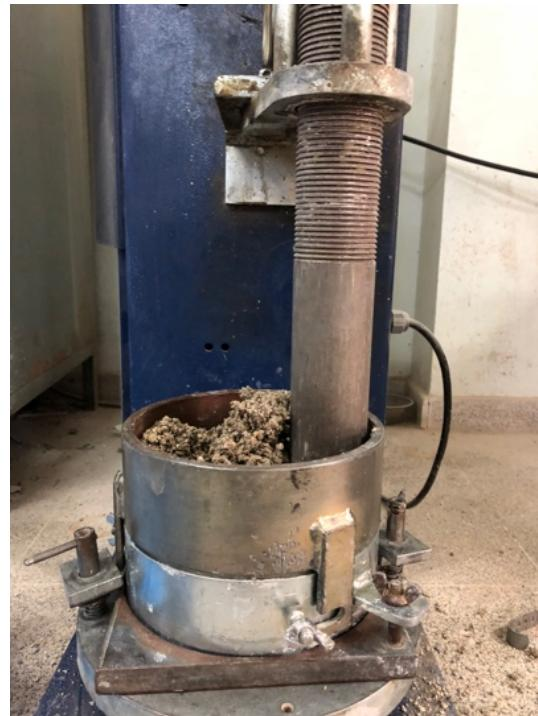
Figure 2.10 The automatic compactor, used for compaction tests (Personal archive, 2017)
