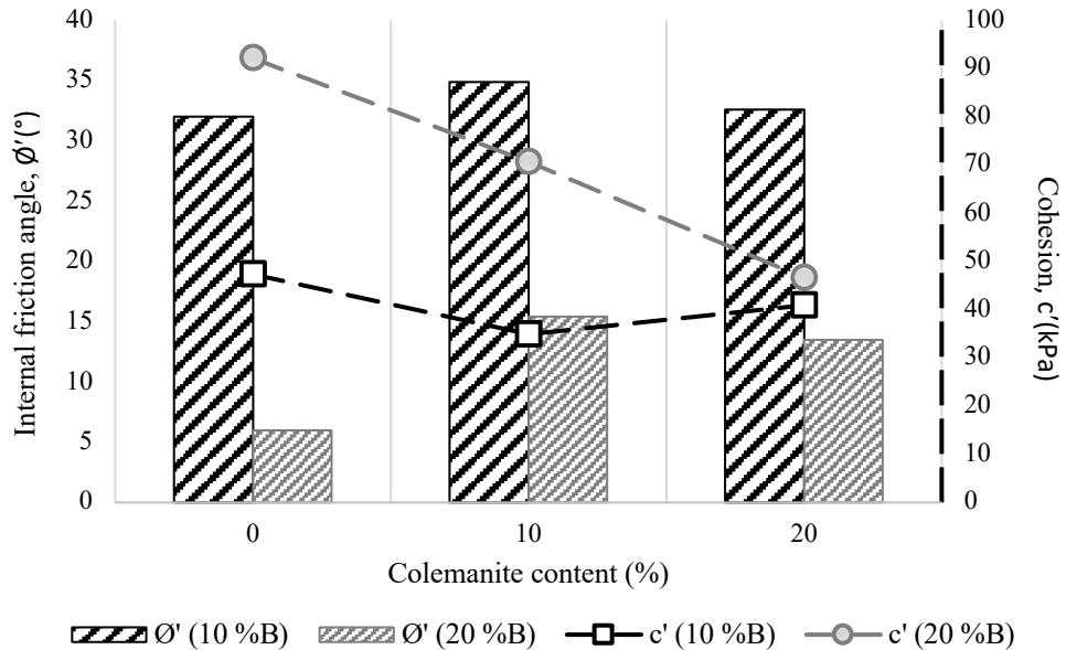
Figure 3.35 Internal friction angle and cohesion values depending on the colemanite percentage of sand-bentonite mixtures at  $80^\circ\text{C}$
