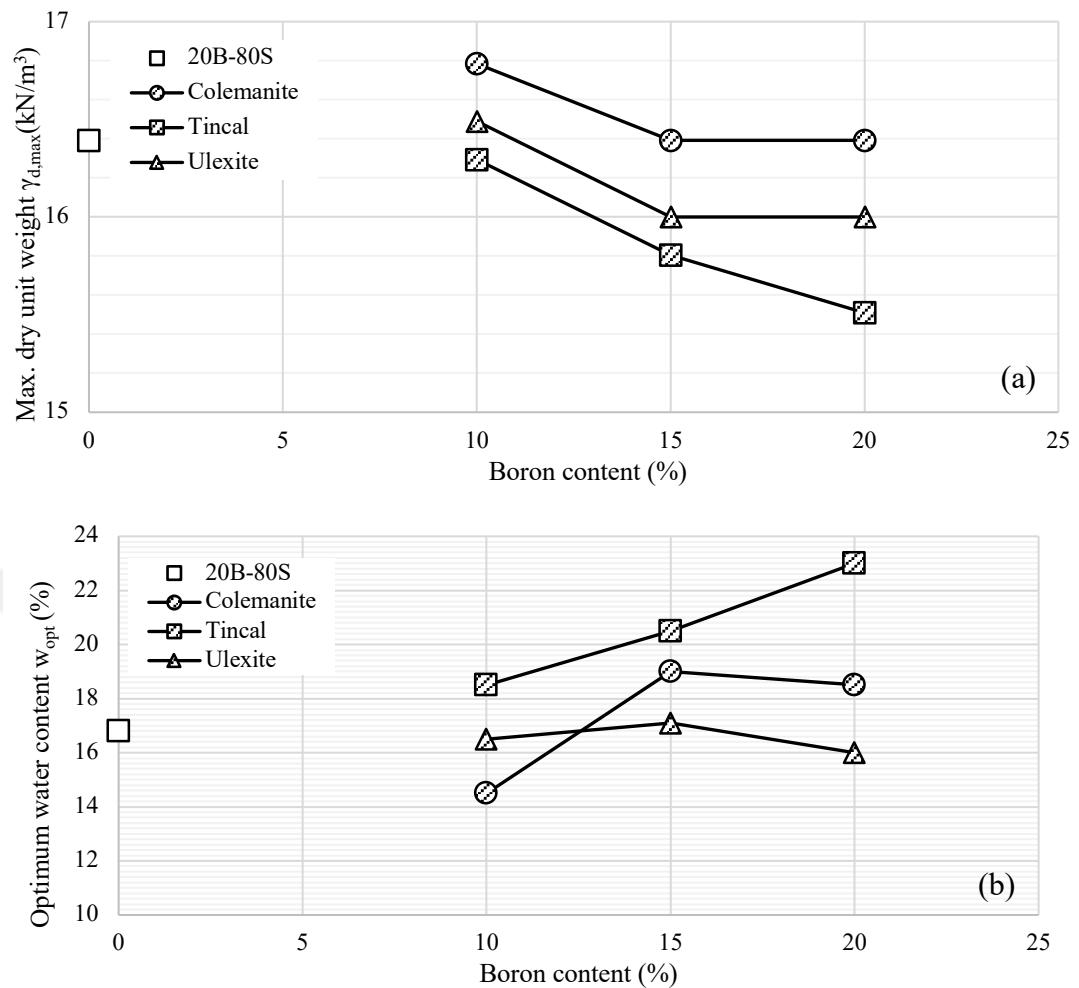
Figure 3.6 Compaction parameters a) max. dry unit weight b) optimum water content of 20% sand-bentonite mixtures in the presence of boron minerals
