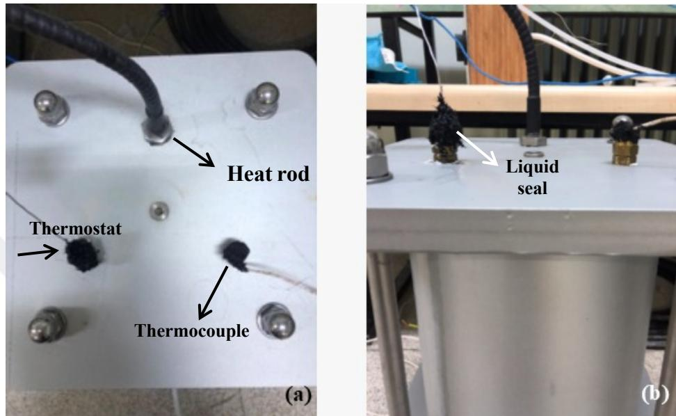
Figure 2.20 Preparation of the modified permeameter a) Insertion of resistance, thermostat and thermocouple in the cell b) application of liquid seal to prevent leakage (Personal archive, 2019)
