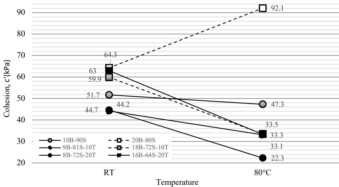
Figure 3.29 Cohesion values of 10% and 20% sand-bentonite mixtures in the presence of tincal at room temperature and at 80°C
