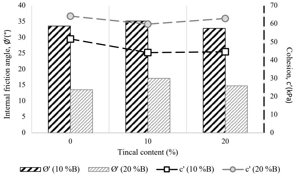
Figure 3.38 Internal friction angle and cohesion values depending on the tincal percentage of sand-bentonite mixtures at room temperature
