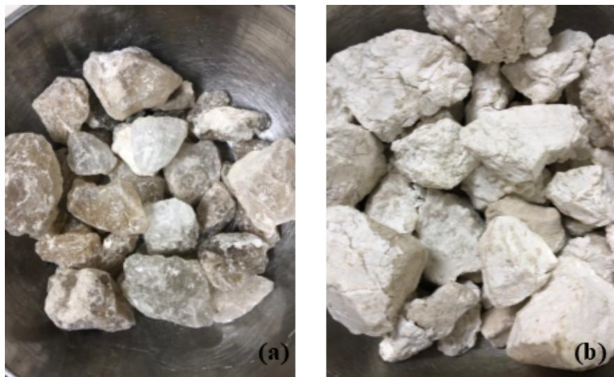
Figure 2.4 Tincal a) at the natural state b) after dry in the oven (Personal archive, 2018)
