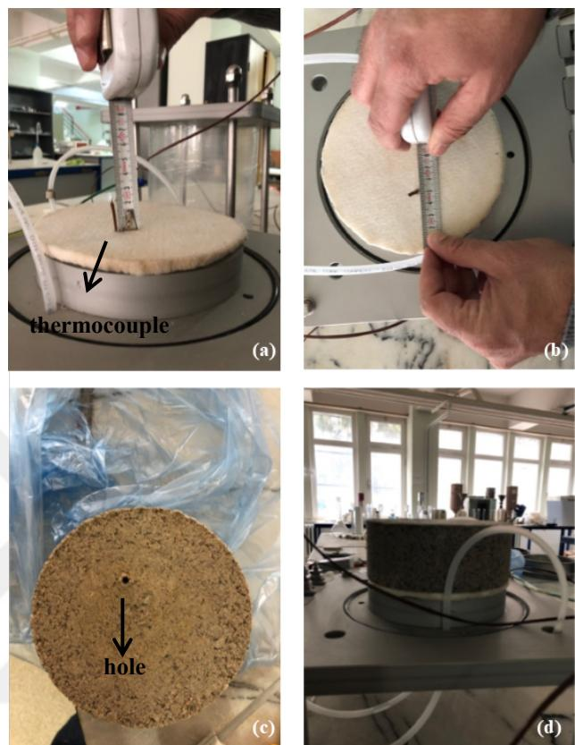
Figure 2.21 Placement of the sample into the permeameters for tests under high temperature a) forming the hole on the geotextile and passing the thermocouple through the hole b) measuring the location of the thermocouple c) forming the hole in line with the thermocouple on the soil d) placing the soil on the thermocouple (Personal archive, 2019)
