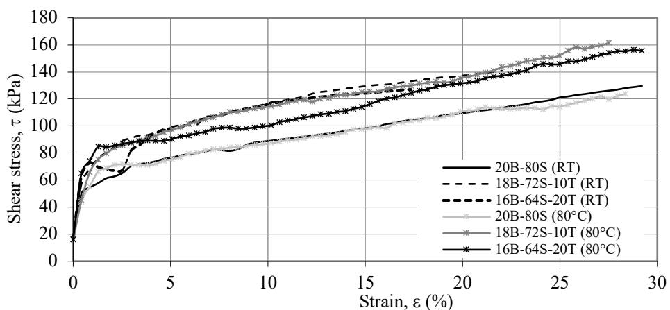
Figure 3.19 The shear stress-strain of 20% sand-bentonite mixtures in the presence of tincal at room temperature and at 80°C
