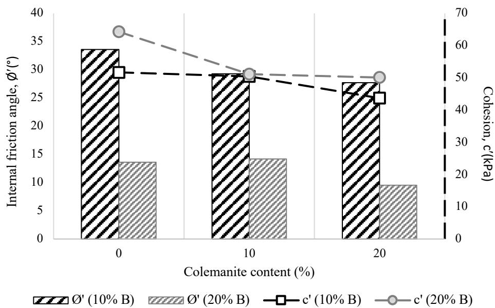
Figure 3.34 Internal friction angle and cohesion values depending on the colemanite percentage of sand-bentonite mixtures at room temperature
