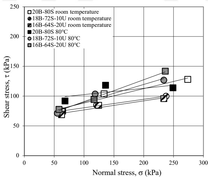
Figure 3.24 The shear failure envelopes of 20% sand-bentonite mixtures in the presence of ulexite at room temperature and at 80°C
