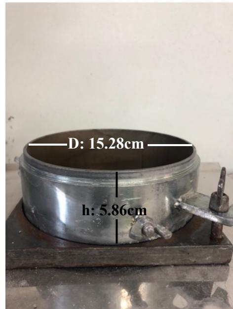
Figure 2.9 Short mold used for compaction tests (Personal archive, 2017)
