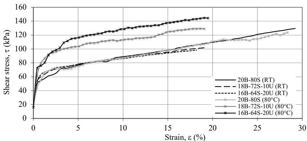
Figure 3.23 The shear stress-strain of 20% sand-bentonite mixtures in the presence of ulexite at room temperature and at 80°C
