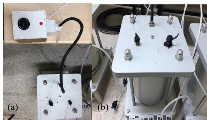
Figure 2.22 Flexible wall permeameter test cells a) thermostat connection b) top view of the cell (Personal archive, 2019)
