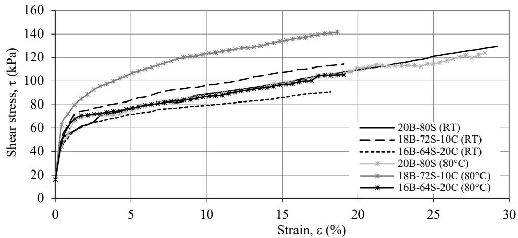
Figure 3.15 The shear stress-strain of 20% sand-bentonite mixtures in the presence of colemanite at room temperature and at 80°C
