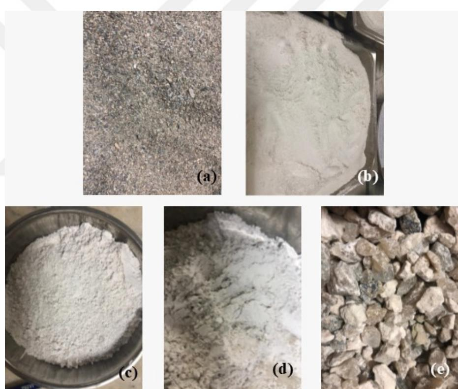
Figure 2.1 Materials used in this study a) sand b) bentonite c) colemanite d) tincal e) ulexite (Personal archive, 2018)
