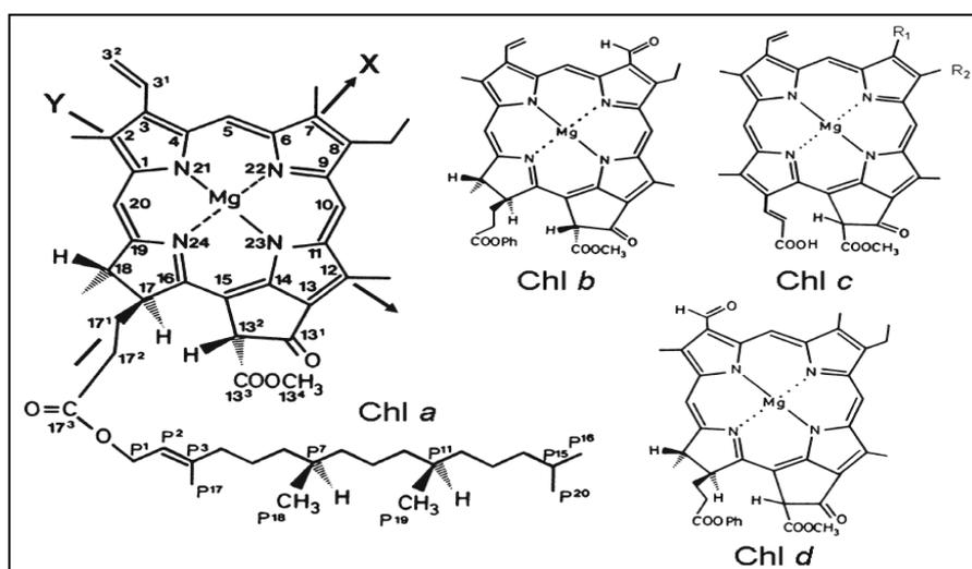
Figure 1.3 Structures of the major chlorophylls. All Chls are tetrapyrroles, where nitrogen atoms are co-ordinated around a Mg atom. Except for the oxidation of the 7-methyl group in Chl *a* to the formyl group in Chl *b*, Chls *a* and *b* are identical. Chl *d* contains a formyl group at position 3. Chl *c*, also contains double bonds in the side chain between positions 17<sup>1</sup> and 17<sup>2</sup> and in the macrocycle between carbons 17 and 18 (Hooper, 2012).
