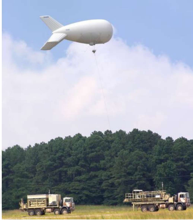
Figure 1.2 Tethered Lighter than Air Aircraft (Raytheon, 2018)
