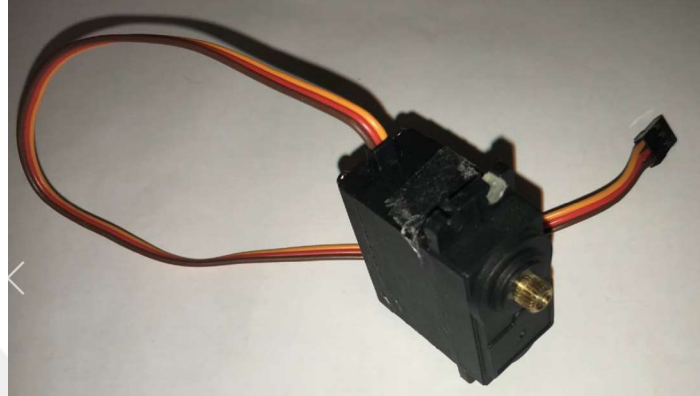
Figure 2.8 TowerPro MG996R Servo Motor (Personal archive, 2018)
