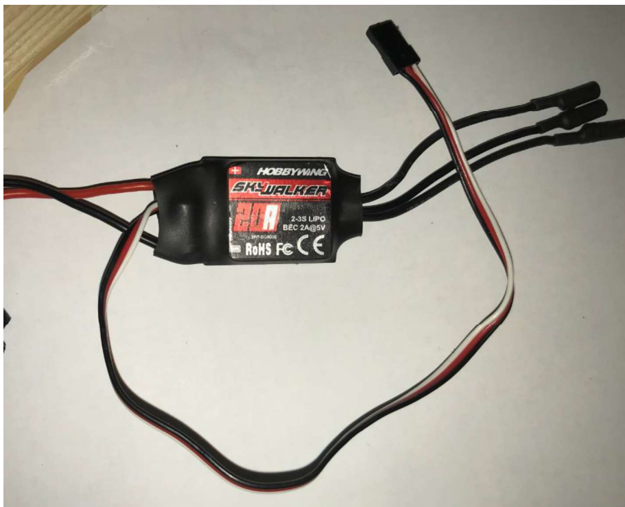
Figure 2.6 Hobbywing Skywalker 20A Electronic speed controller (Personal archive, 2018)
