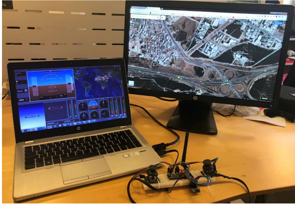
Figure 2.56 Ground Control Module prototype (Personal archive, 2018)
