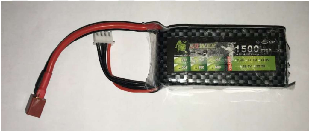
Figure 2.7 3S, 11,1V, 1500mah Li-Po Battery (Personal archive, 2018)
