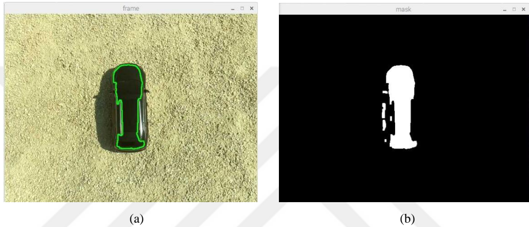
Figure 2.25 Object (car) detection in center position (a) Real frame of target (b) Masked image of target
