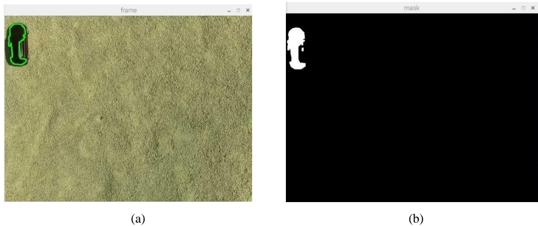
Figure 2.26 Object (car) detection in left-forward diagonal position (a) Real frame of target (b) Masked image of target
