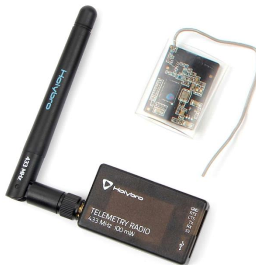
Figure 2.11 Telemetry module transceivers (Holybro, 2019)
