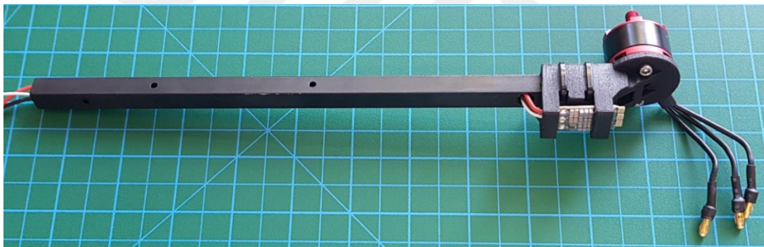
Figure 2.17 Aluminium arm of the UAV (Personal archive, 2019)
