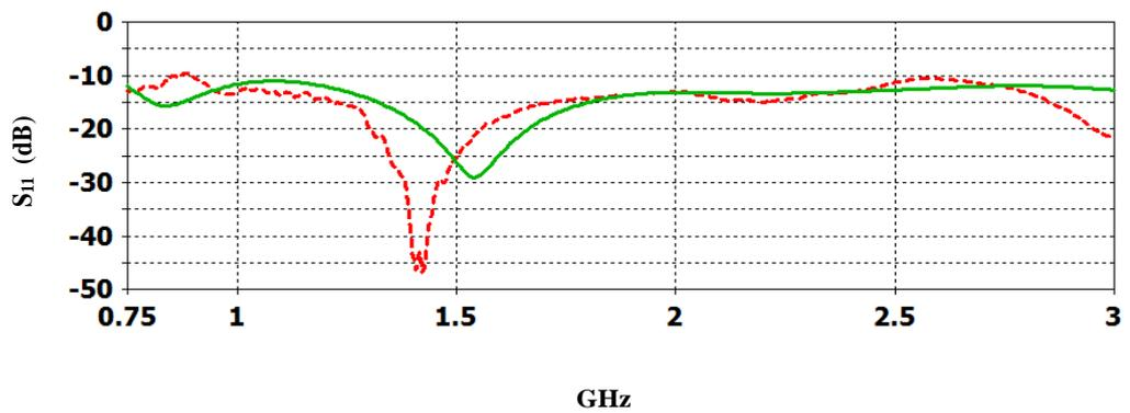
Figure 3.7 Comparison of measured and simulated  $S_{11}$  for the printed circular disc planar monopole antenna (--- measurement, — simulation)
