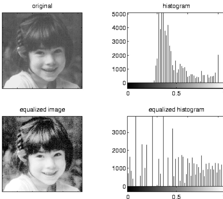
Figure 3.1 The original image and its histogram, and the equalized versions. Both images are quantized to 64 grey levels.
