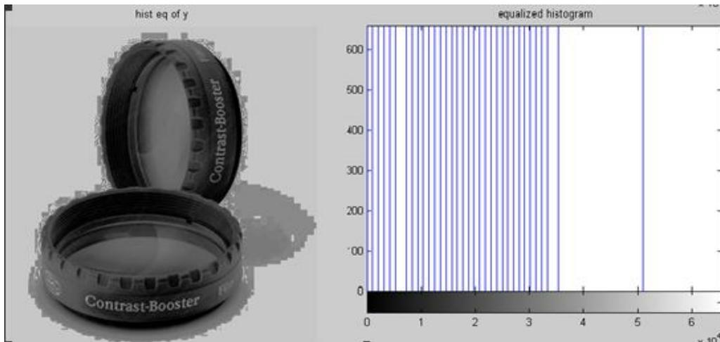
Figure 3.3 Standard HE applied to image and its histogram with “histeq” command
