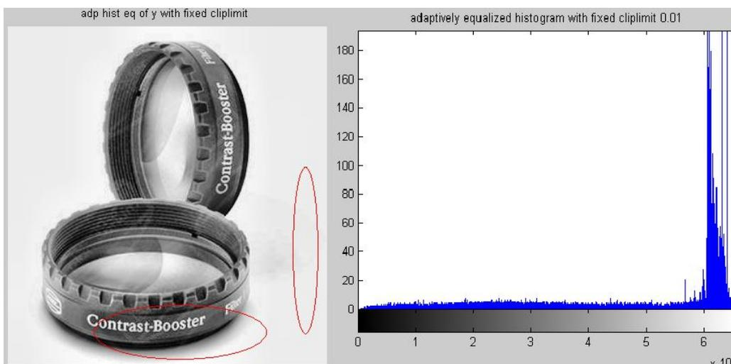
Figure 3.4 AHE applied to image and its histogram with “Adaphstheq” command by fixed clip limit 0.01
