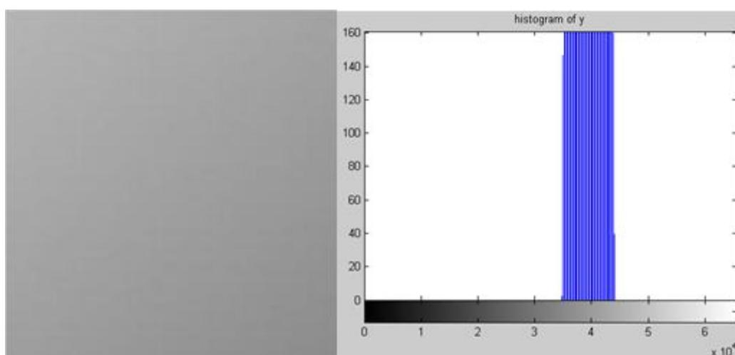
Figure 2.12 Image and its histogram after typical contrast algorithm
