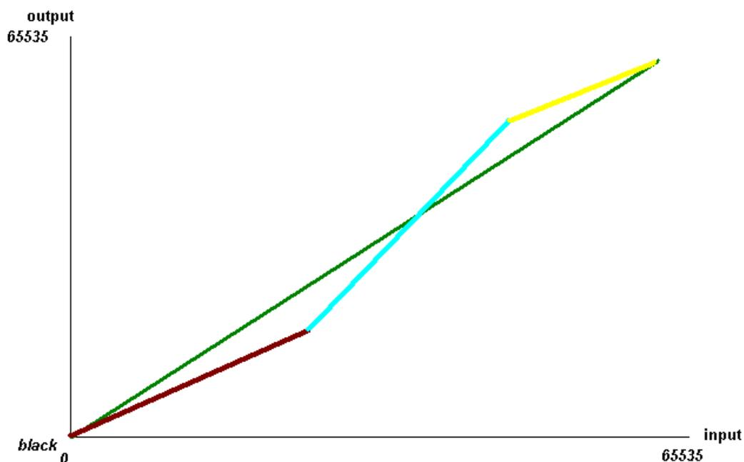
Figure 2.2 Typical contrast algorithm with 3 segments
