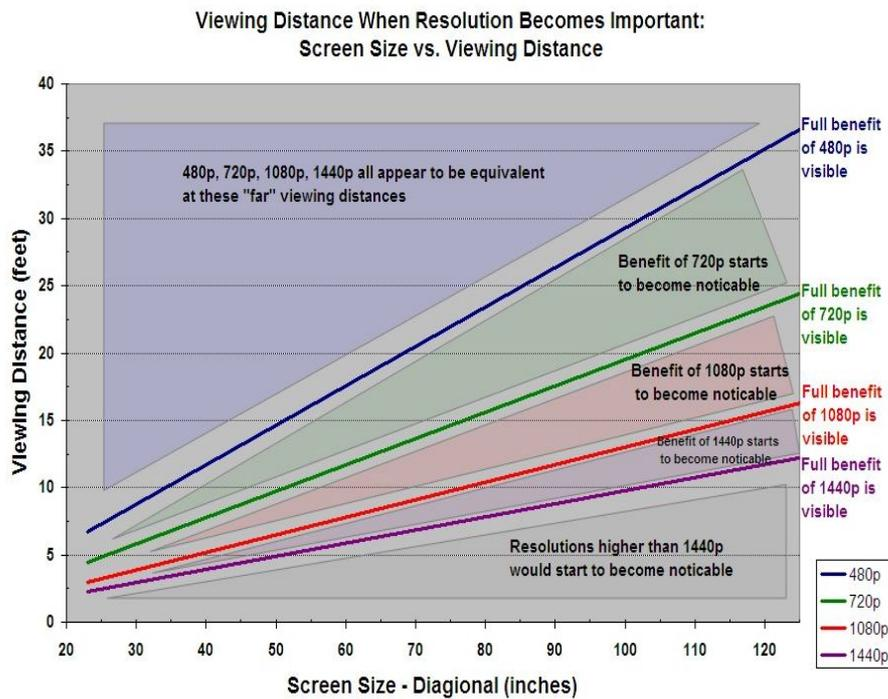
Figure 5.18 viewing distance depending to screen and image resolution
