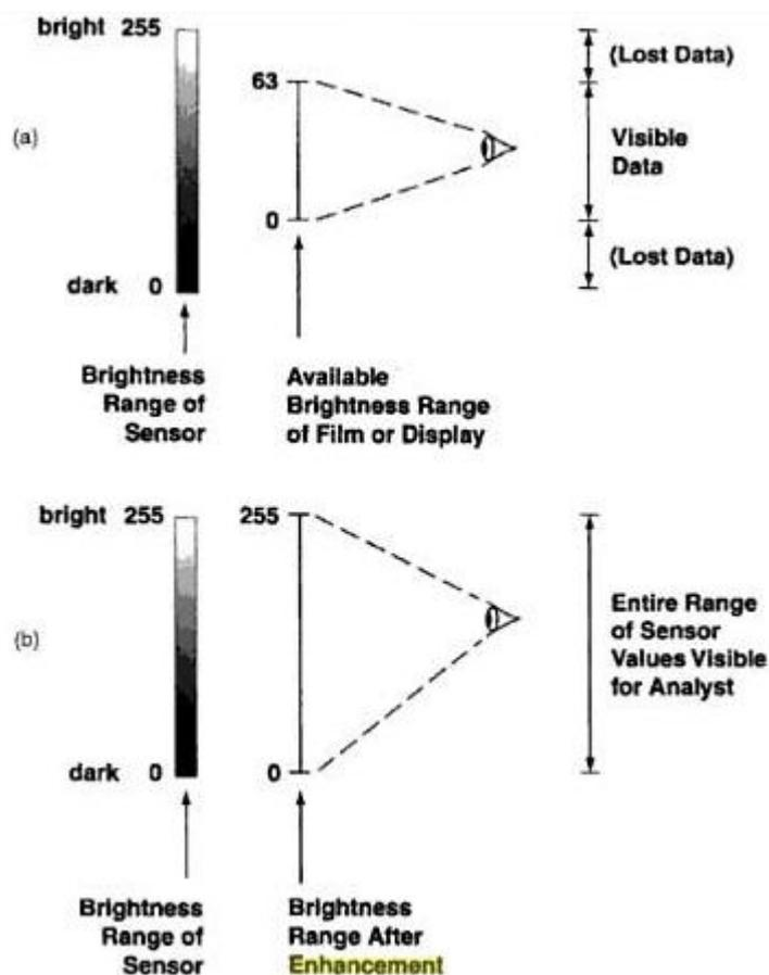
Figure 2.1 Loss of visual data in display of digital image
