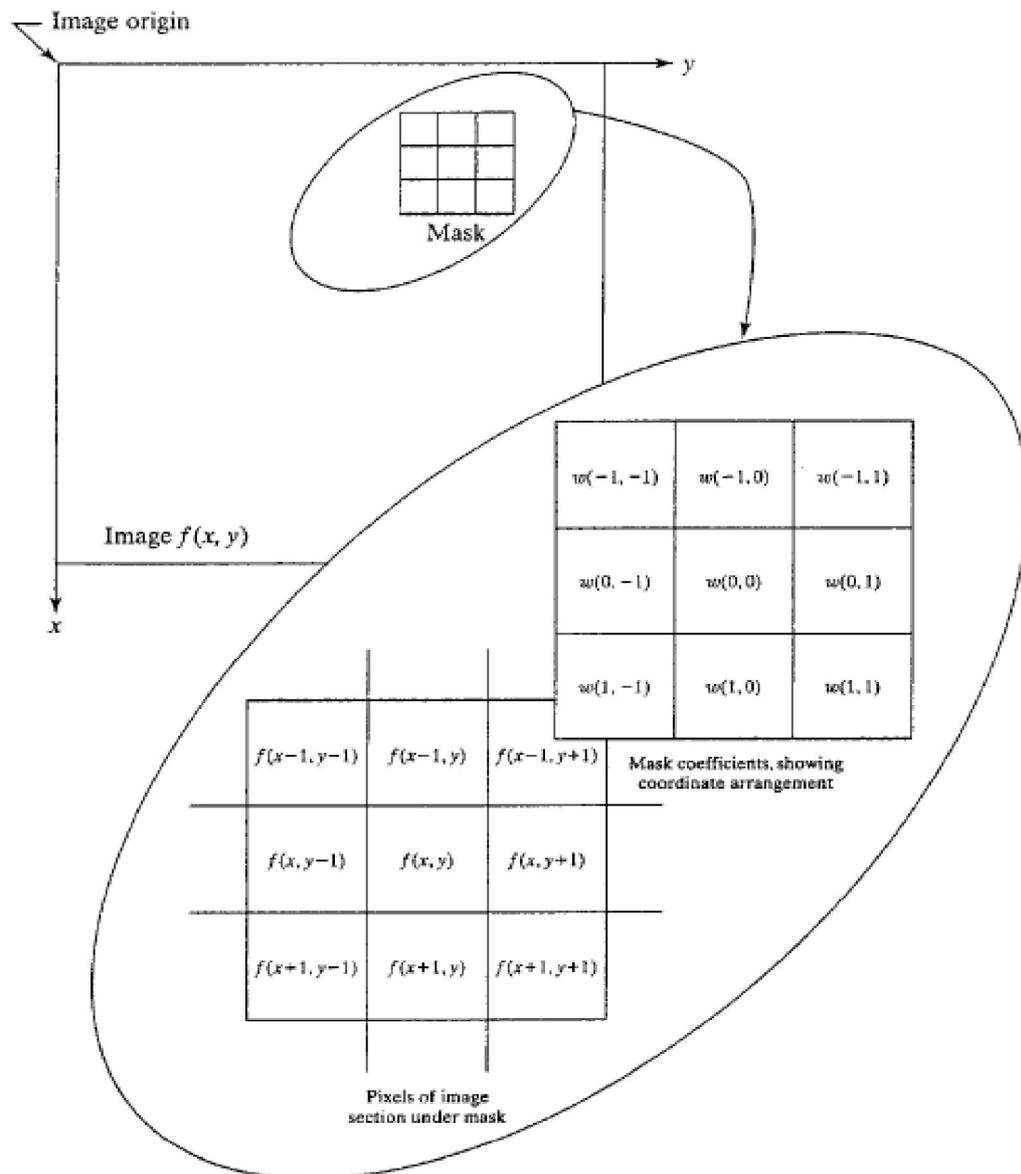
Figure 4.4 The mechanics of spatial filtering
