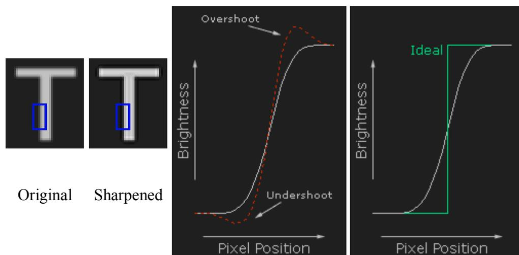
Figure 4.5 The response of sharpness algorithm in image
