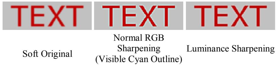
Figure 4.5 The response of sharpness algorithm in image
